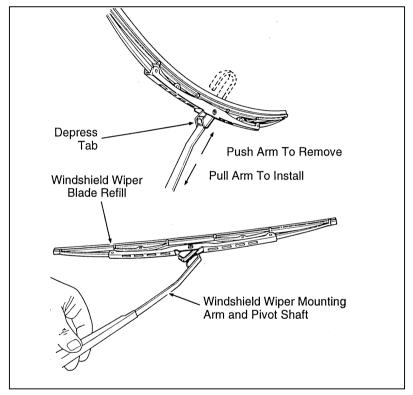
Replacing the wiper blades
