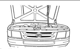
While applying upward pressure on the hood, lift the auxiliary latch release handle and raise the hood. Insert support rod in hood prop hole. To close, raise hood slightly and remove support rod from the prop hole. Slam hood shut. After closing, always make sure your hood is latched securely by trying to lift it.
