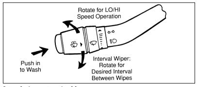
Interval wiper on turn signal lever
