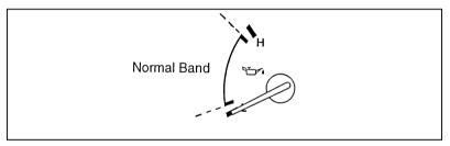
Engine oil pressure gauge — mechanical cluster
