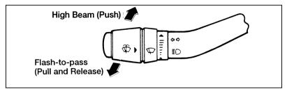
Headlamp high beam switch and turn signal lever on steering column
