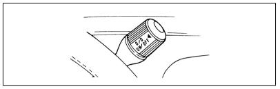
Transmission control switch (located on the end of the gearshift lever)
