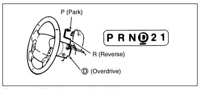
The positions of the column-mounted gearshift
