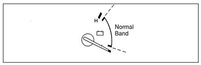
Battery voltage gauge — mechanical cluster
