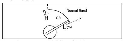
Battery voltage gauge — mechanical cluster with tachometer
