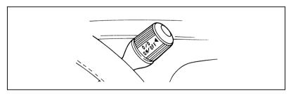
Transmission control switch (located on the end of the gearshift lever)
