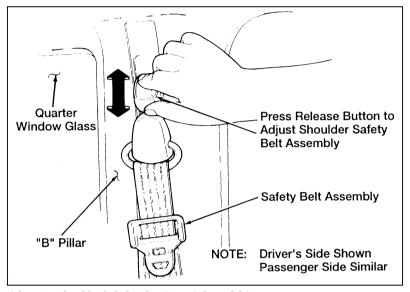
Adjusting shoulder belt height (SuperCab models)
