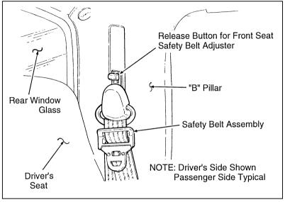
Shoulder belt height adjuster — full down position (regular cab models)
