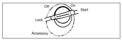
The positions of the key in the ignition lock cylinder.
