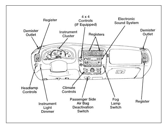
The main controls for the climate control system, lights, lamps, clock, and radio are on the instrument panel.
