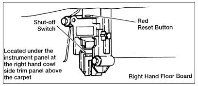
Fuel pump shut-off switch location
