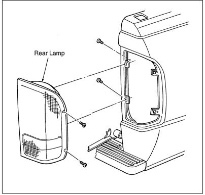
Replacing the tail lamp bulb
