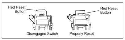
Reset button for fuel pump shut-off switch
