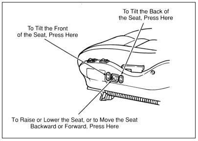
The power controls on the driver's seat
