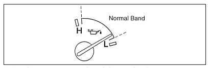
Engine oil pressure gauge — mechanical cluster with tachometer
