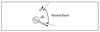
Engine coolant temperature gauge — mechanical cluster
