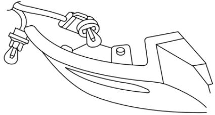
5. Pull the bulb from the socket and push in the new bulb.
