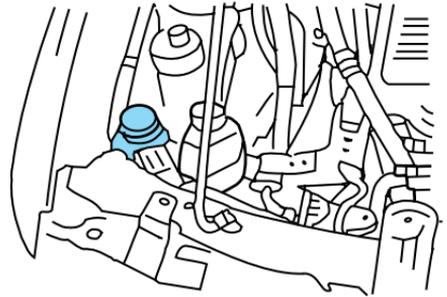
Check the level of the engine coolant in the reservoir. Refer to the Scheduled Maintenance Guide for service interval schedules. Be sure to read and understand *Precautions when servicing your vehicle* in this chapter.
