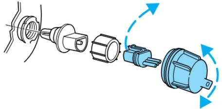
4. Release clip and disconnect the electrical connector from the bulb.
