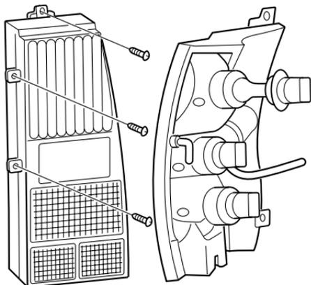
1. Open liftgate to expose the tail lamp assembly. Remove the three screws and lamp assembly from the vehicle.
