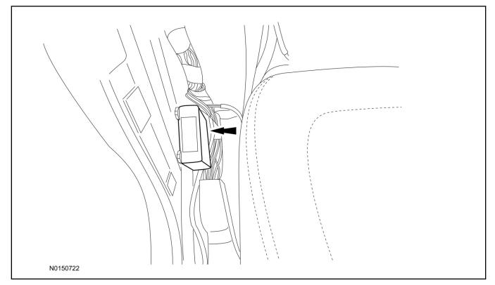
10. Connect the female end of the 8-pin T-harness to the TPM module.
