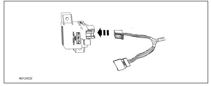
20. Connect the male end of the 8-pin T-harness to the vehicle's existing TPM module harness.
