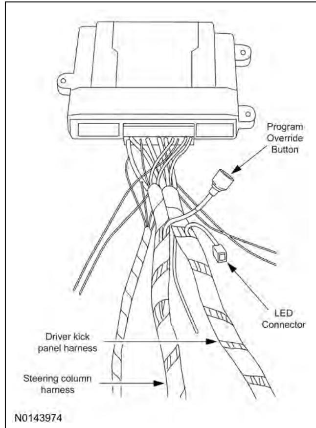
7. Tape the harness sections together, making sure to cover all of the unused wires.
