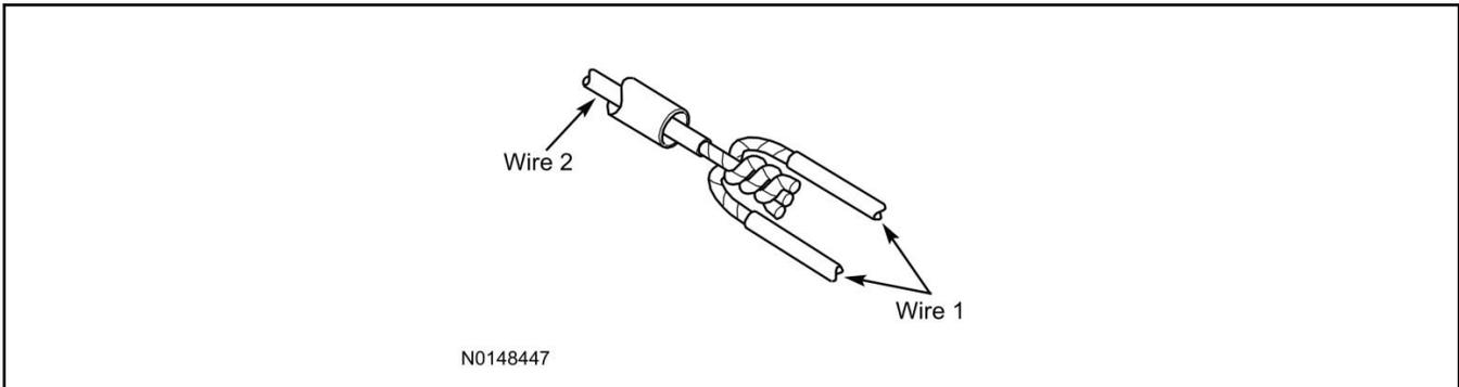
**17. Evenly position heat shrink tubing over wire repair.**
