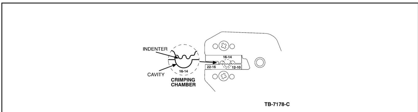
9. Center one (1) end of the butt splice on the appropriate crimping chamber. If visible, be sure to place the brazed seam of the butt splice toward the indenter. Hold the butt splice in place and squeeze the tool handles together until the ratchet engages sufficiently to hold the butt splice in position (typically one (1) or two (2) clicks). DO NOT deform the butt splice. Insert stripped wire into the butt splice, making sure the insulation on wire does not enter the butt splice.
