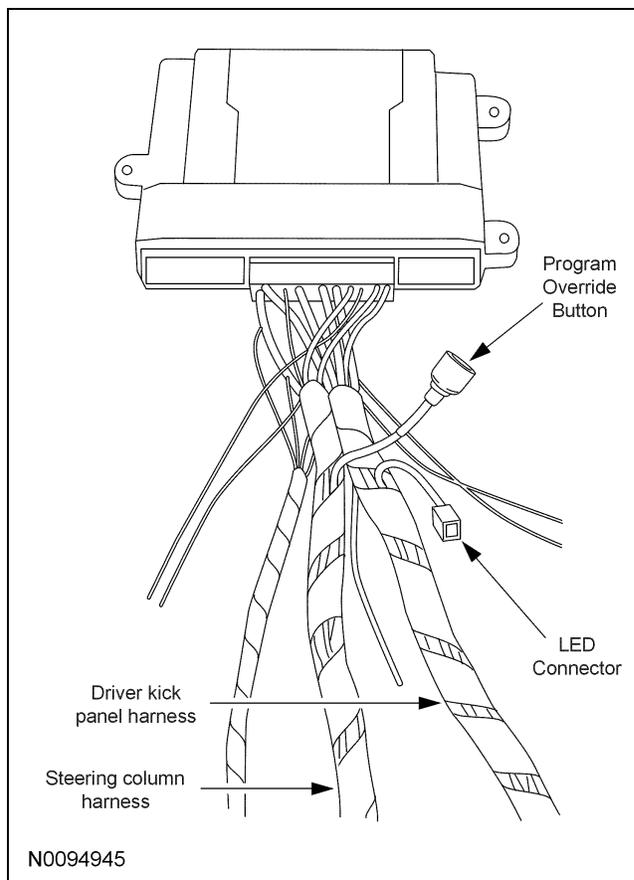
8. Tape the harness sections together, making sure to cover all of the unused wires.
