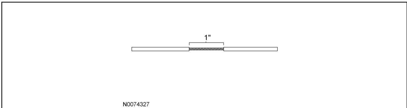
3. On the vehicle wire to be spliced into, separate the strands to allow the new wire to be placed.
