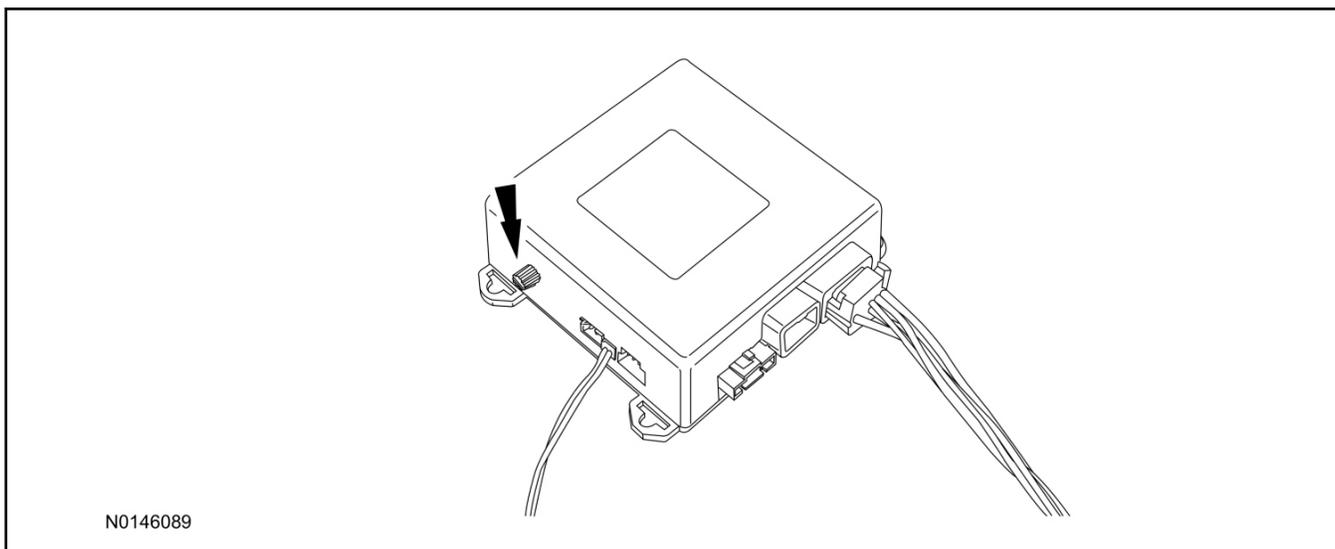
14. Starting with the adjustment knob in approximately the halfway position, lower the driver's window and exit the vehicle.
