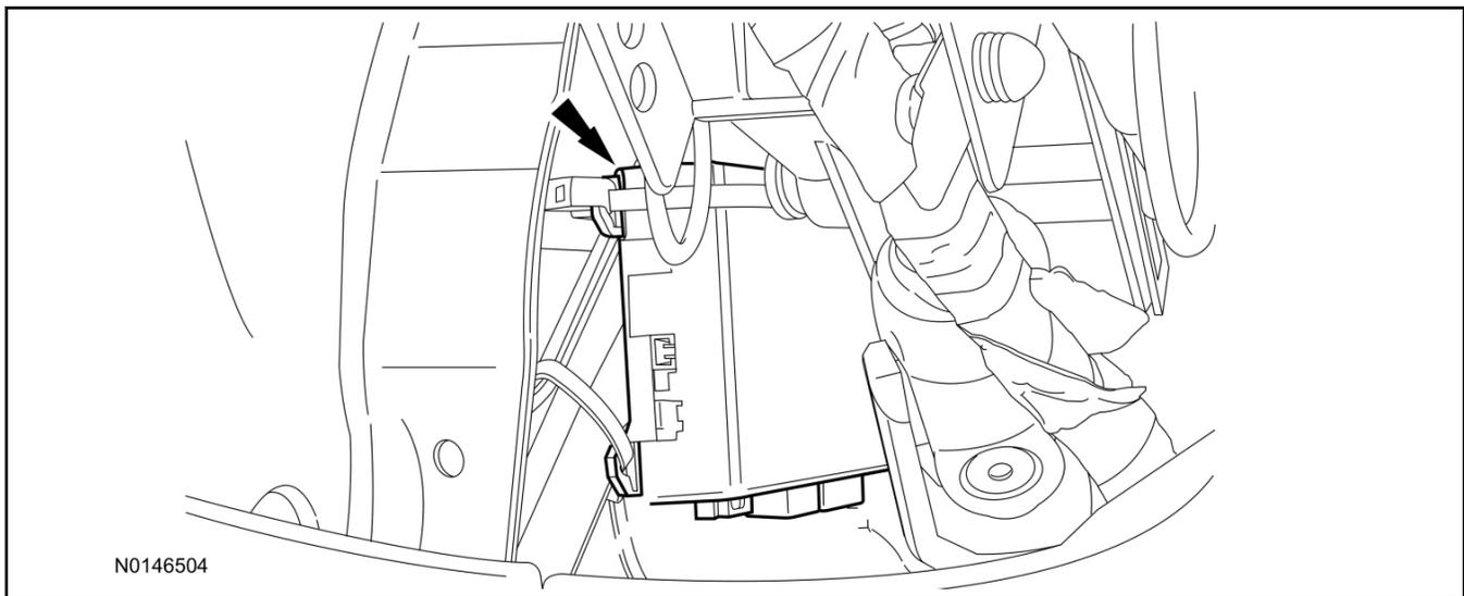
7. Position the T-harness inside the IP.
