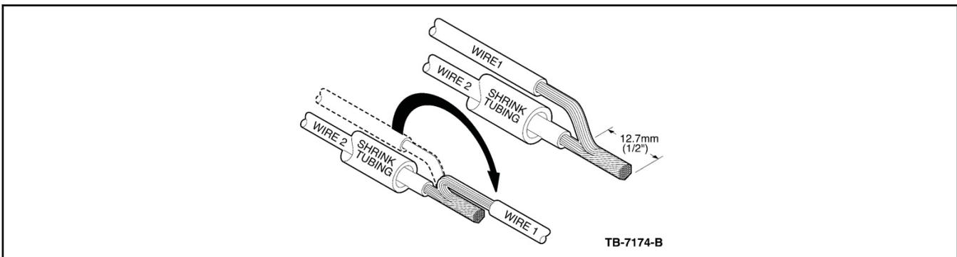
**3-Wire Solder Splice Procedure**
