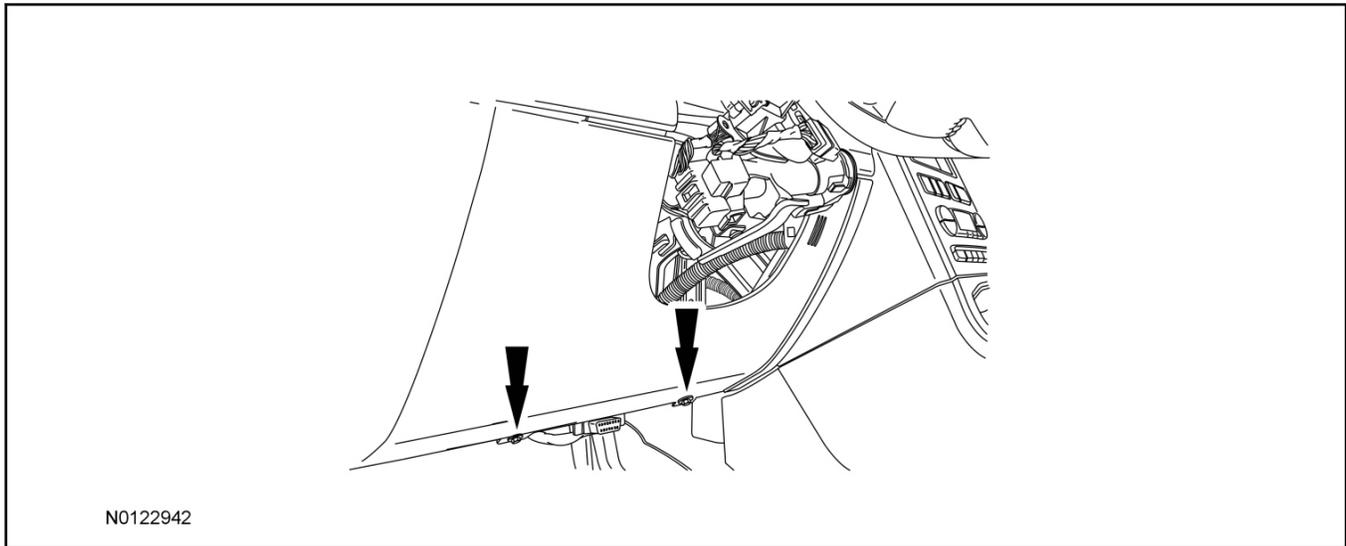
11. If equipped, disconnect the electrical connector and hose from the temperature sensor.
