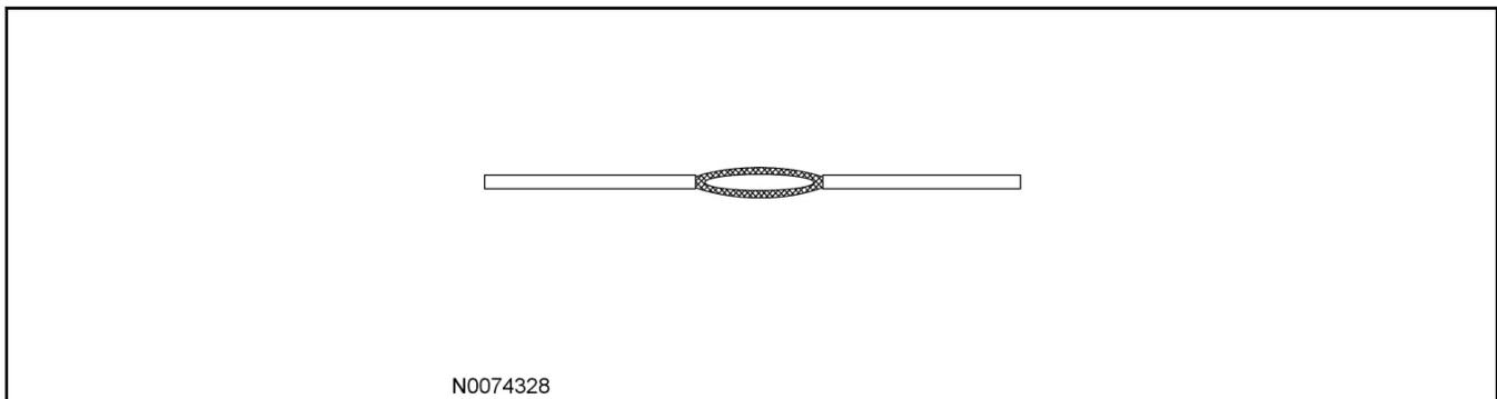
4. Insert the new wire between the parted strands. If more than one wire is being spliced, wrap them in opposite directions.
