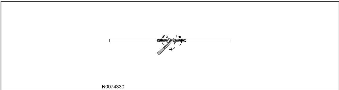
6. Wrap the connection with electrical tape so the tape covers the wires approximately two inches on either side of the connection.
