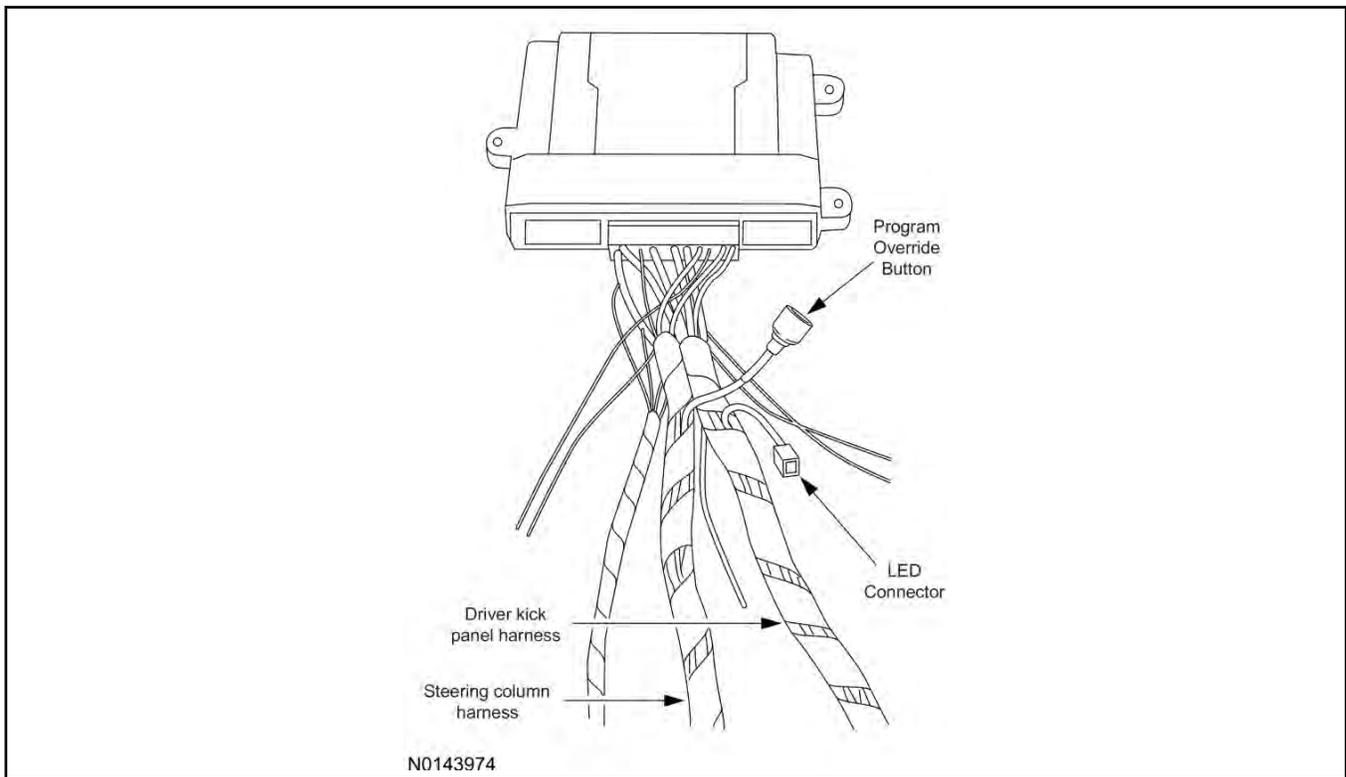
7. Tape the harness sections together, making sure to cover all of the unused wires.
