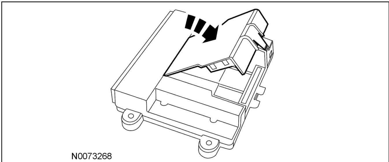
5. Plug the wiring harness(es) into the module.
