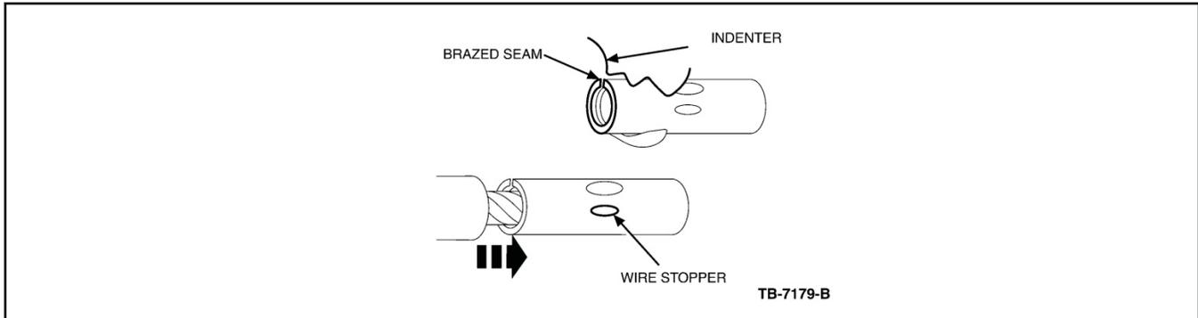
10. Holding the wire in place, squeeze tool handles together until ratchet releases. Allow tool handles to open, then remove crimped butt splice.
