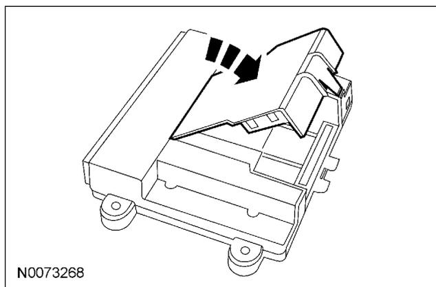
5. Plug the wiring harness(es) into the module.
