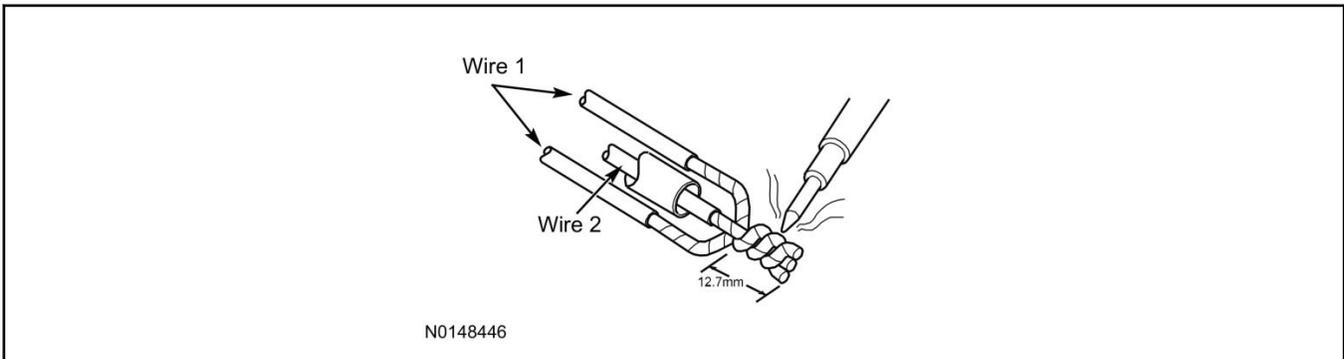
**16. Bend Wire #1 back over the twisted wires for sealing. Inspect solder joint bond.**
