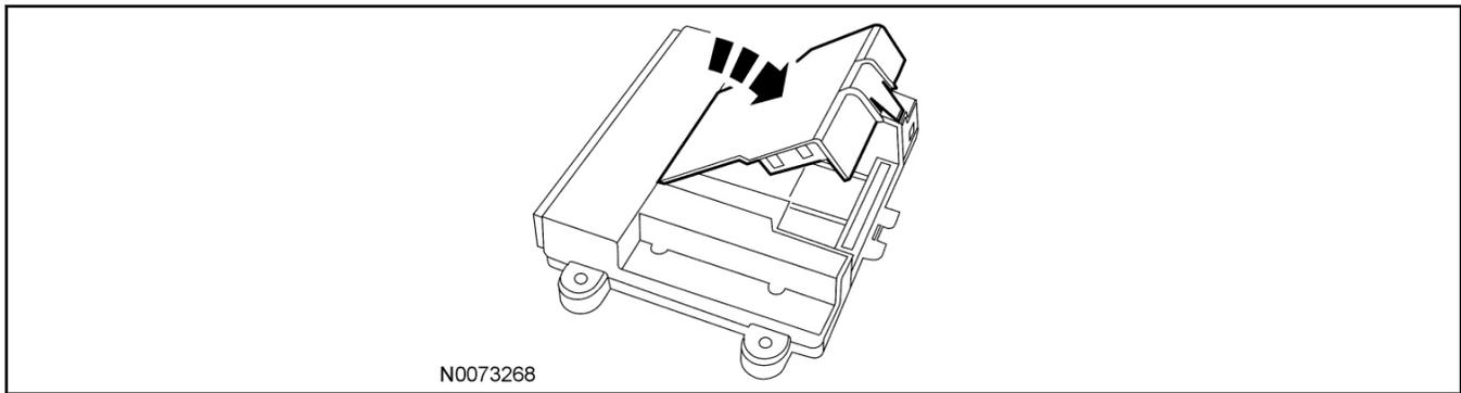
5. Plug the wiring harness(es) into the module.
