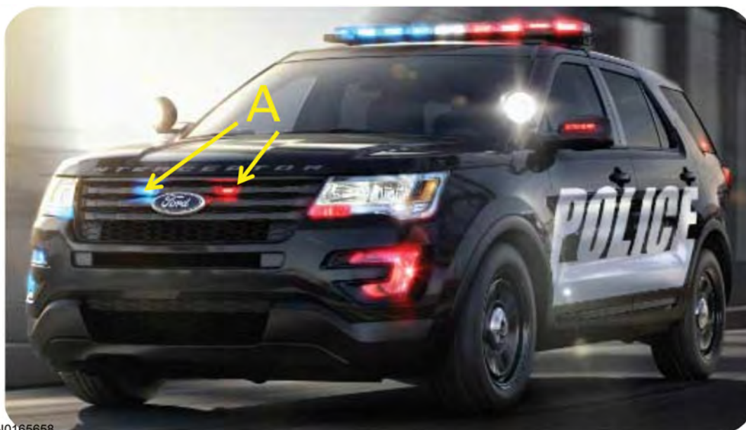
A. Integrated LED grille lights
