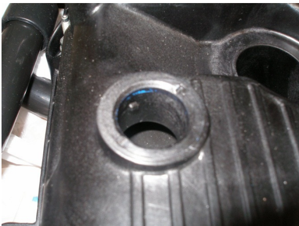
Rocker cover with nub for quarter-turn valve
