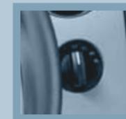
**4X4 AUTO** mode provides electronic control four-wheel drive with power delivered to all four wheels, as required, for increased traction.
