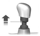
**Note:** The gearshift lever can only be moved to **R** (Reverse) by raising the collar below the gearshift knob up before shifting to reverse. This is a lockout feature which protects the transmission from accidentally engaging **R** (Reverse) when intending to select 1 (First).
