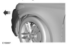
Separate the front bumper cover from the fender, pull the fender outward 3 cm.
