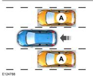
BLIS aids you in detecting vehicles that may have entered the blind spot zone (A). The detection area is on both sides of the vehicle, extending rearward from the exterior mirrors to approximately 10 feet (3 meters) beyond the bumper. The system alerts you if certain vehicles enter the blind spot zone while driving.
