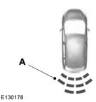
A Coverage area of up to 6 feet (2 meters) from the rear bumper.
