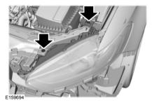
4. Remove the two headlamp assembly screws.
