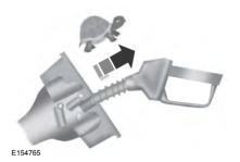
4. After you are done pumping fuel, slowly remove the fuel filler nozzle—allow about five to ten seconds after pumping fuel before removing the fuel filler nozzle. This allows residual fuel to drain back into the fuel tank and not spill onto the vehicle.
