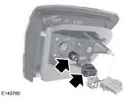
7. Remove the bulb from the bulb holder. Install the new bulb in reverse order.
