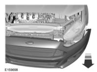
8. From the front of the vehicle, pull the front bumper cover forward 10 cm.
