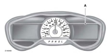
The display is located on the right side of your instrument cluster. You can use your steering wheel controls to view and make minor adjustments to active modes without taking your hands off the wheel. For example:
