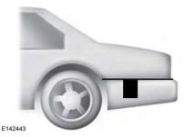
The system uses radar sensors which are located behind the bumper fascia on each side of your vehicle. Do not allow these areas to become obstructed by mud, snow or bumper stickers, as this can cause degraded system performance.
