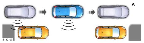
When a suitable space is found, the touch screen displays a message and a chime sounds. Slow down and stop at approximately position (A), then follow the instructions on the touch screen.
