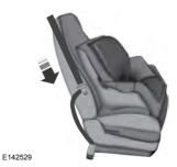
2. Pull down on the shoulder belt and then grasp the shoulder belt and lap belt together.
