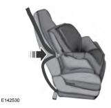
While holding the shoulder and lap belt portions together, route the tongue through the child seat according to the child seat manufacturer's instructions. Be sure the belt webbing is not twisted.
