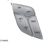
The cruise controls are located on the steering wheel.
