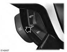
The cruise controls are located on the steering wheel.
