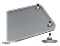
To install floor mats, position the floor mat so that the eyelet is over the retention post and press down to lock in.
