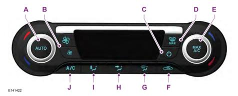
A **AUTO** and **Driver temperature control:** Press the button to turn on automatic operation. Select the desired temperature using the temperature control. The system adjusts fan speed, air distribution, air conditioning operation, and selects outside air or recirculated air to heat or cool the vehicle in order to maintain the desired temperature. You can also use the **AUTO** button to turn off dual zone operation by pressing and holding the button for more than two seconds.
