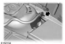
4. Make the final connection of the negative (-) cable to an exposed metal part of the stalled vehicle's engine, or connect the negative (-) cable to the ground connection point, if available.
