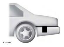
The system uses radar sensors that are located behind the bumper fascia on each side of your vehicle. Do not allow mud, snow or bumper stickers to obstruct these areas, this can cause degraded system performance.
