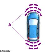
A Coverage area of up to 27 inches (70 centimeters) from the front of the vehicle and about 14 inches (35 centimeters) to the side of the front end of the vehicle. Refer to the reverse
