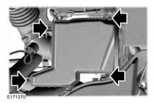
1. Loosen the four fasteners and remove the air cleaner assembly lid.
