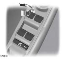
Press the control to open the window. Lift the control to close the window.
