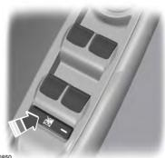
Press the control to lock or unlock the rear window controls. It lights when the rear window controls lock.
