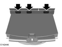
Vehicles with the standard size spare tire can adjust the load floor to two positions. The front of the load floor can be placed either on (for high position) or below (for low position) the ledges behind the rear seats. The rear of the load floor always sits on the two small shelves located on the liftgate trim.
