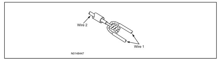
4. Evenly position heat shrink tubing over wire repair.
