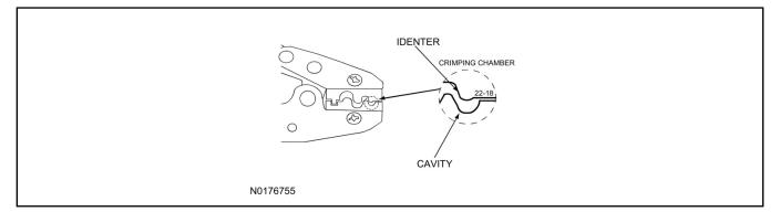
3. Center one (1) end of the butt splice on the appropriate crimping chamber. If visible, be sure to place the brazed seam of the butt splice toward the indenter. Hold the butt splice in place and squeeze the tool handles together until the ratchet engages sufficiently to hold the butt splice in position (typically one (1) or two (2) clicks). DO NOT deform the butt splice. Insert stripped wire into the butt splice, making sure the insulation on wire does not enter the butt splice.
