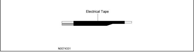
2-Wire Solder Splice/Ratcheting Crimp Tool Splice Procedure
