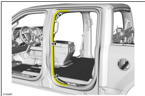
23. Release the clips and disengage the safety belt pretensioner boot from the pretensioner bezel.
