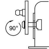
Rotate the bolt 90° to align tailgate fastener notches with edges of the slot.
