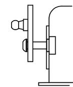
Pull out on lower ball mount plate to engage tailgate fastener into slot.
