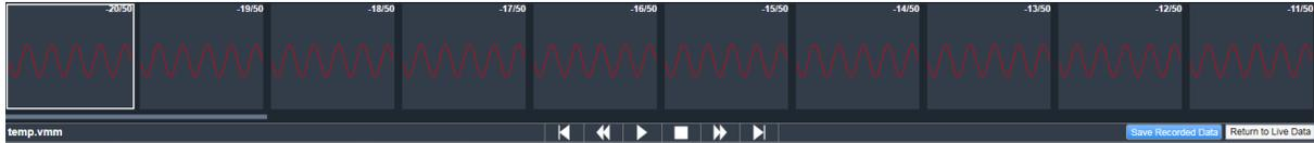
Three mini-images are shown in the example below. This timeline was created with a Record Setting of “Record From” = 20, and a “Record Length” = 50. The frame with the white border is the active frame, which is shown in full resolution in the main view. The sequence number of this frame is -20/50. The value of -20 means the frame was recorded 20 frames before the “Start Recording” button was pressed. The value of 50 means a total of 50 frames were recorded.
