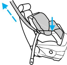
8. Allow the safety belt to retract to remove any slack in the belt.
