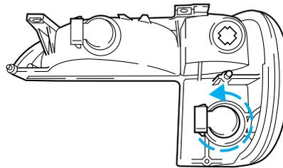
8. Carefully pull bulb straight out of socket and push in the new bulb.
