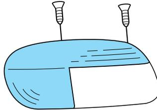
7. Rotate bulb socket counterclockwise and remove from lamp assembly.
