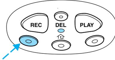
The 2nd or 3rd press from step 3 will activate the door. The HomeLink® Universal Transceiver has now been trained to the receiver. The remaining two buttons may now be programmed if this has not previously been done.
