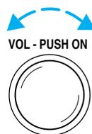
If the volume is set above a certain level and the ignition is turned off, the volume will come back on at a “nominal” listening level when the ignition switch is turned back on. If you wish to maintain your preset volume level, turn the audio system off with the power control before switching off the ignition.
