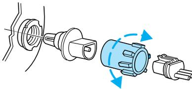
4. Remove the old bulb from the lamp assembly by gently pulling it straight back out of the lamp assembly.
