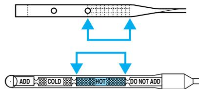
The transmission fluid should be in this range if at ambient temperature (10°C-35°C [50°F-95°F]).
