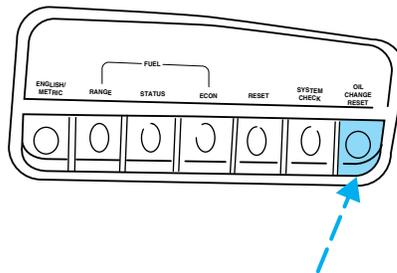
Your personalized oil reset percentage allows you to establish a smaller oil change interval than the manufacturer's recommended interval. To establish your personalized oil reset percentage:
