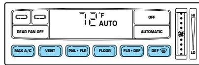
The air conditioning compressor will operate in all modes except FLOOR and VENT. It will also operate only when required when AUTOMATIC has been selected. However, the air conditioning will only function if the outside temperature is about 6°C (43°F) or higher.
