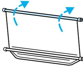
4. Push in the right end cap (marked RH) about  $\frac{1}{4}$  of the total length to disengage the clutch and hold the end cap in while turning the roller tube toward you 14 times.
