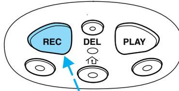
The indicator light will flash amber and an “error” tone will sound if the **REC** button is pressed when memory is full.
