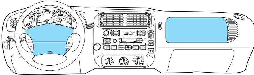
Your vehicle is equipped with a crash sensing and diagnostic module which records information about the air bag and sensor systems. In the event of a collision this module may save information related to the collision including information about the air bag system and impact severity. This information will assist Ford in the servicing of your vehicle and may help Ford better understand real world collisions and further improve the safety of future vehicles.
