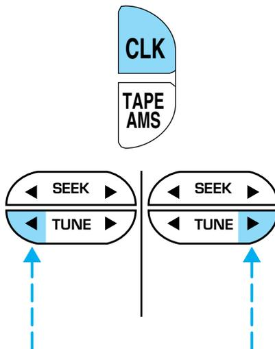
The CLK control will allow you to switch between media display mode (radio station, stereo information, etc.) and clock display mode (time).
