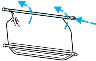
5. Let go of the right end cap. The clutch will now engage and stop the shade from losing its spring tension.
