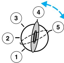
3. If the temperature is below  $-12^{\circ}\text{C}$  ( $10^{\circ}\text{F}$ ) and the engine does not start in 15 seconds on the first try, turn the key OFF and wait 10 seconds and try again. If the engine does not start in two attempts, press the accelerator pedal all the way to floor and hold. Turn the key to START position.
