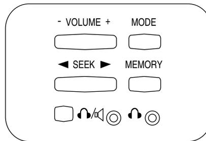
To turn on the rear seat controls, press the memory preset controls 3 and 5 at the same time. The
