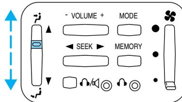
The instrument panel climate controls must be on in order for the rear console climate controls to work.
