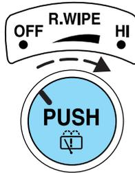
Press the control for rear washer fluid operation.
