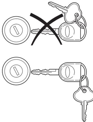
momentary concern if they are too close to the key during engine start. If a problem occurs, turn ignition OFF and restart the engine with all other objects on the key ring held away from the ignition key. Check to make sure the encoded ignition key is an approved Ford encoded ignition key.
