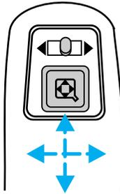
3. Return to the center position to lock mirrors in place.
