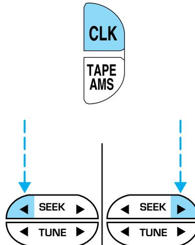
To set the minute, press and hold the CLK control and press the TUNE control:
