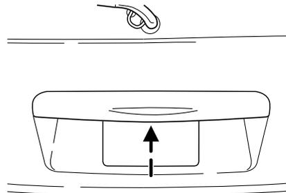
To lock the liftgate and the liftgate window, use the key or the power door locks, depress the key lock cylinder or press the door lock switch on the left side of the cargo area.
