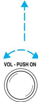
If the volume is set above a certain level and the ignition is turned off, the volume will come back on at a “nominal” listening level when the ignition switch is turned back on.
