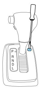
If it is necessary to use the above procedure to move the gearshift lever, it is possible that a fuse has blown or the vehicle's brakelamps are not operating properly. Refer to *Fuses and relays* in the *Roadside Emergencies* chapter.
