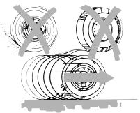
Your vehicle has anti-lock brakes, therefore apply the brakes steadily. Do not "pump" the brakes.
