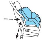
10. Try to pull the belt out of the retractor to make sure the retractor is in the automatic locking mode (you should not be able to pull more belt out). If the retractor is not locked, unbuckle the belt and repeat Steps 2 through 9.
