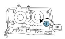
5. Discard the old bulb and install the new bulb into bulb socket.
