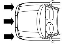
wrong with the system. Rather, it means the forces were not of the type sufficient to cause activation. Front airbags are designed to activate in frontal and near-frontal collisions, not rollover, side-impact, or rear-impacts unless the collision causes sufficient longitudinal deceleration.
