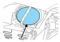
• The filter can be accessed from the first row seat. Move the front seats all the way back and up to ease access.
