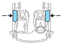
• Two crash sensors located under the outboard side of the front seats, attached near the floor.
