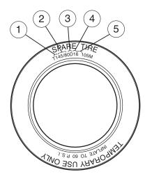
of the tire in millimeters from sidewall edge to sidewall edge. In general, the larger the number, the wider the tire.
