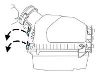
careful not to crimp the filter element edges between the air filter housing and cover. This could cause filter damage and allow unfiltered air to enter the engine if not properly seated.
