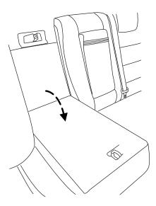
Before returning the seatback to its original position, make sure that cargo or any objects are not trapped behind the seatback. After returning the seatback to its original position, pull on the seatback to ensure that it has fully latched. An unlatched seat may become dangerous in the event of a sudden stop or collision.
