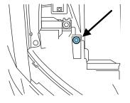
HORIZONTAL AIM IS NOT REQUIRED FOR THIS VEHICLE AND IS NON-ADJUSTABLE.
