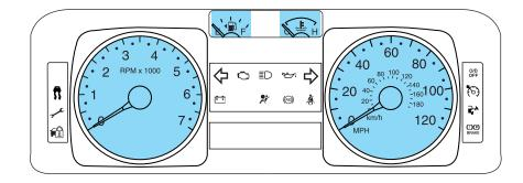
**Speedometer:** Indicates the current vehicle speed.
