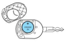
2. Do not wipe off any grease on the battery terminals on the back surface of the circuit board.
