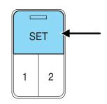
2. Within five seconds, press any control on the Integrated Keyhead Transmitter which you would like to deactivate and then press the SET control on the driver's door panel again.
