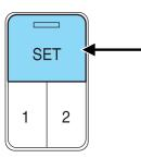
Press the SET control. The SET control light will briefly illuminate. While the light is illuminated, press control 1.
