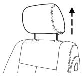
Push release button to lower head restraint.
