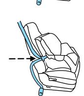
4. Insert the belt tongue into the proper buckle (the buckle closest to the direction the tongue is coming from) for that seating position until you hear a snap and feel the latch engage. Make sure the tongue is latched securely by pulling on it.
