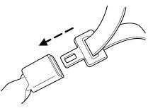
2. To unfasten, push the release button and remove the tongue from the buckle.
