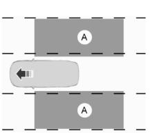
BLIS® aids the driver in detecting vehicles that may have entered the blind spot zone (A). The detection area is on both sides of the vehicle, extending rearward from the exterior mirrors to approximately 10 feet (3 meters) beyond the bumper. The system alerts you if certain vehicles enter the blind spot zone while driving.
