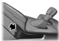
1. Using a screwdriver (or similar tool), carefully pry off and remove the BSI access panel.
