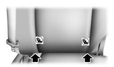
The LATCH anchors are located at the rear section of the rear seat between the cushion and seatback below the symbols as shown. Follow the child seat manufacturer's instructions to properly install a child seat with LATCH attachments.
