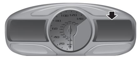
The display is located on the right side of your instrument cluster. You can use your steering wheel controls to view and make minor adjustments to active modes without taking your hands off the wheel. For example:
