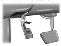
1. Inside the vehicle, pull the hood release handle located under the bottom of the instrument panel near the steering column.
