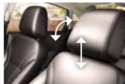
**Note:** Do not force the head restraint backward after it is tilted. Instead, continue tilting it forward until the head restraint releases to the upright position.
