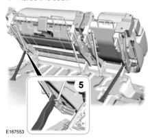
5. Lift the support rod and connect it to the seat frame. This prevents the seat from falling backward.
