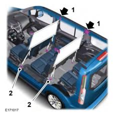
1. Push the ends of the upper bar toward each other and insert them into the retainers in the roof. Push the bar forward into the narrow section of the retainers.
