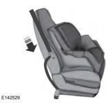
2. Pull down on the shoulder belt and then grasp the shoulder belt and lap belt together.
