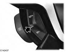
The cruise control switches are located on the steering wheel.
