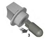
Remove the bulb by pulling it straight out.
