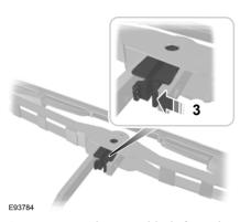
3. Disengage the wiper blade from the wiper arm.
