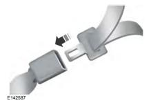
Insert the safety belt tongue into the proper buckle (the buckle closest to the direction the tongue is coming from) until you hear a snap and feel it latch. Make sure the tongue is securely fastened in the buckle.
