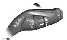
Push the lever away from you to operate the rear window washer. When you release the lever, wiping continues for a short period of time.
