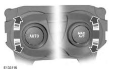
You can set the temperature between 60°F (15.5°C) and 85°F (29.5°C). In position LO, the system switches to permanent cooling. In position HI, the
