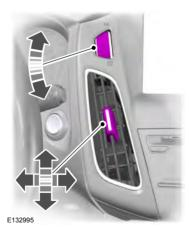
To close the air vent, turn the thumbwheel above the vent fully downward.
