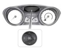
You can use the information display control on the steering wheel to adjust various system settings on your vehicle. The instrument panel will display the system settings.
