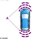
A The front parking aid sensor coverage area is up to 31 inches (80 centimeters) from the center of your vehicle's front bumper and up to 14 inches (35 centimeters) to the side of your vehicle's front bumper. The rear parking aid sensor coverage area is up to 72 inches (183 centimeters) from the center of your vehicle's rear bumper. There is a decreased coverage area at
