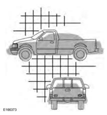
As a result of the above dimensional differences, sport-utility vehicles, vans and trucks often will have a higher center of gravity and a greater difference in center of gravity between the loaded and unloaded condition.
