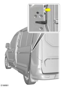
The childproof locks are located on the rear edge of each rear door and must be set separately for each door.
