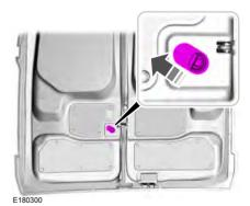
Slide the release lever up to open the door in an emergency.
