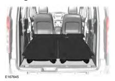
The carpeted cover is held in position by magnets. Fold the carpeted cover forward to cover up the folded seats.
