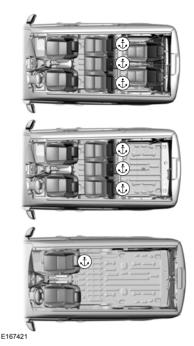
Perform the following steps to install a child safety seat with tether anchors:
