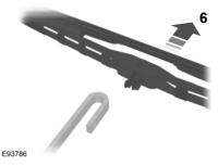
6. Remove the wiper blade. Install new wiper blades in the reverse order.
