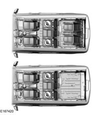
Your vehicle has LATCH lower anchors for child seat installation at the seating positions marked with the child seat symbol.
