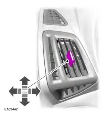
To close the air vent, slide the airflow direction control fully downward.
