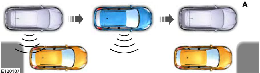
When a suitable space is found, the touch screen displays a message and a chime sounds. Slow down and stop at approximately position (A), then follow the instructions on the touch screen.
