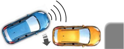
When automatic steering is finished, the touch screen displays a message indicating that the active park assist process is done. The driver is responsible for checking the parking job and making any necessary corrections before putting the transmission in P (Park).
