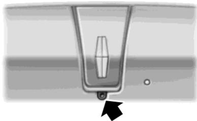
The camera is located on the liftgate.
