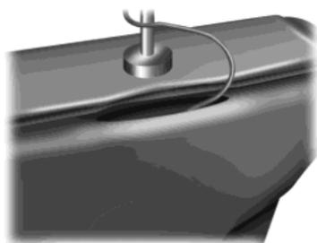
When in use, place the rear outboard safety belts in the comfort guides. These guides are attached to the head restraint and are stored in a pocket in the seat back.
