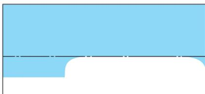
On the wall or screen you will observe a flat zone of high intensity light located at the top of the right hand portion of the beam pattern. If the top edge of the high intensity light zone is not at the horizontal reference line, the headlamp will need to be adjusted.
