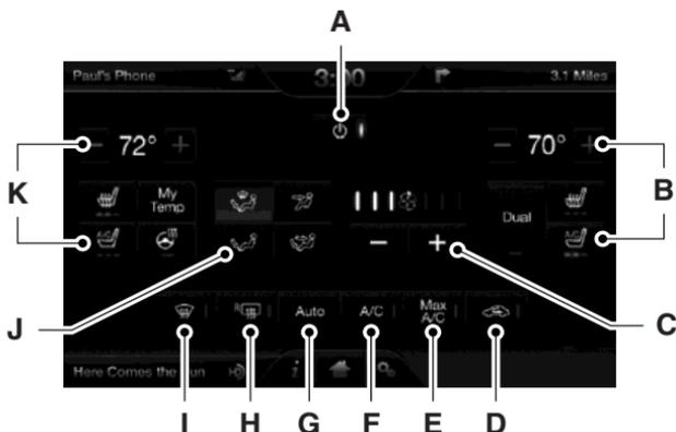
A. **Power:** Touch to switch the system off and on. Switching off the climate control system prevents outside air from entering the vehicle.
