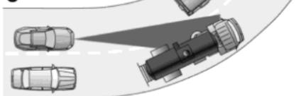
C. There may be issues with the detection of vehicles in front when driving into and coming out of a bend or curve in the road.
