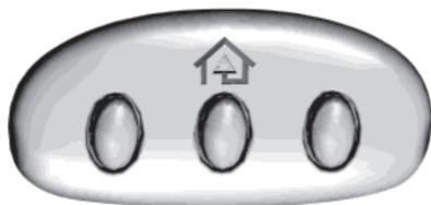
The universal garage door opener replaces the common hand-held garage door opener with a three-button transmitter that is integrated into the driver's sun visor.
