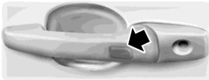
Press and hold the lock sensor area for about a second to lock your vehicle. To avoid unlocking the door inadvertently, make sure to only touch the lock sensor and not other areas of the door handle.
