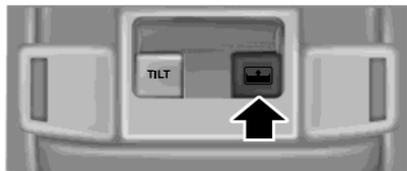
Press and release the control to open the sunshade. The front and rear sunshades open simultaneously.
