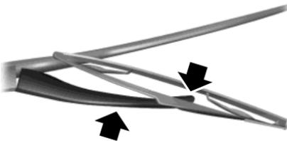
1. Grab the wiper arm with one hand close to the arm/blade joint and pull it as far away from the glass as possible. Do not use excessive force because it can break the wiper arm at the heel. Hold it there until the next step.
