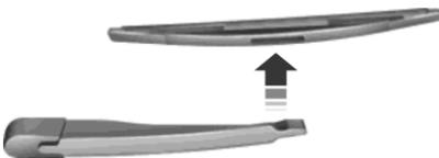
4. Attach the new wiper to the wiper arm and press it into place until a click is heard.
