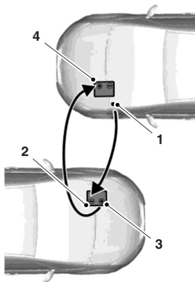
1. Remove the jumper cable from the ground metal surface.
