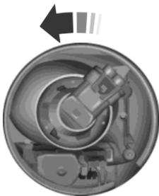
4. Turn the bulb holder counterclockwise and remove it.
