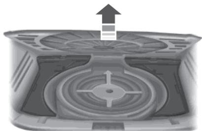
The system is located in the floor of the cargo area. Lift the release handle to open.
