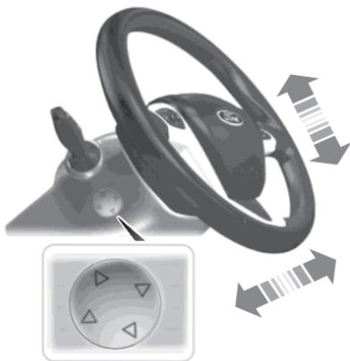
Use the control on the side of the steering column to adjust the position.
