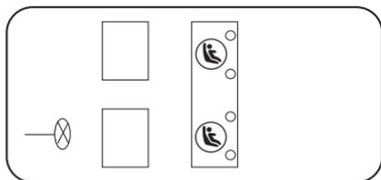
Your vehicle has LATCH lower anchors for child seat installation at the seating positions marked with the child seat symbol.
