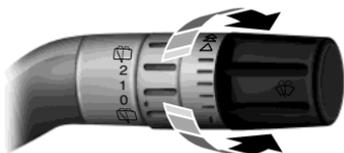
Rotate the end of the control away from you to increase the speed of the wipers. Rotate toward you to decrease the speed of the wipers.
