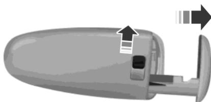
The intelligent access key also contains a removable mechanical key blade that you can use to unlock the driver door. Slide the release on the back of the transmitter to release the mechanical key blade, and then pull the blade out.
