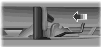
2. Go to the front of the vehicle and release the secondary hood latch located under the front passenger side of the hood.
