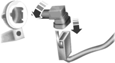
2. From underneath the vehicle, remove the splash shield and rotate the harness/bulb assembly counterclockwise, to remove from the fog lamp.
