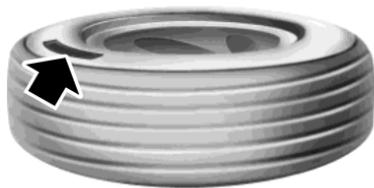
Tire Quality Grades apply to new pneumatic passenger car tires. The Tire Quality Grades can be found where applicable on the tire sidewall between tread shoulder and maximum section width. For example:
