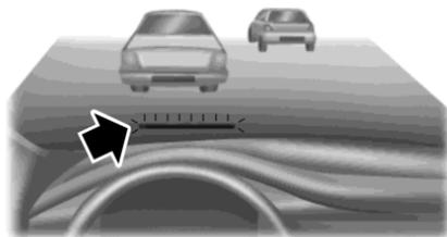
This system is designed to alert the driver of certain collision risks. A radar detects if your vehicle is rapidly approaching another vehicle
