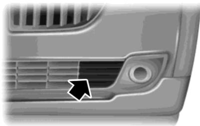
If a message regarding a blocked sensor appears in the information display, the radar signals from the sensor have been obstructed. The sensors are located behind a fascia cover near the driver side of the lower grille. When the sensors are obstructed, a vehicle ahead cannot be detected and the collision warning system does not function. The following table lists possible causes and
