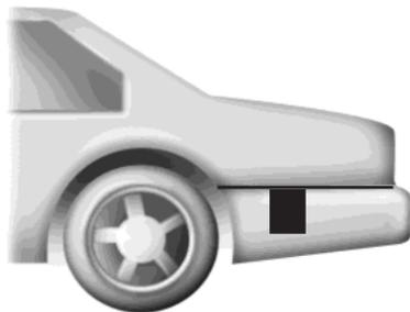
The system uses radar sensors which are located behind the bumper fascia on each side of the vehicle. Do not allow these areas to become obstructed by mud, snow or bumper stickers, as this can cause degraded system performance.
