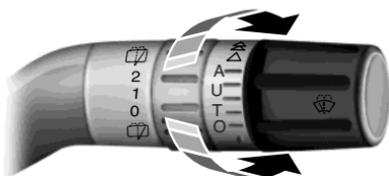
Use the rotary control to adjust the sensitivity to one of the interval moisture settings. The wipers will not cycle until moisture is detected on the windshield. The wiper speed will vary based on the amount of moisture detected on the windshield and the sensitivity setting. The
