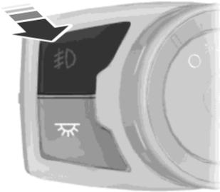
The fog lamps can be turned on when the lighting control is in the headlamps, parking lamps or autolamps positions and the high beams are not turned on.
