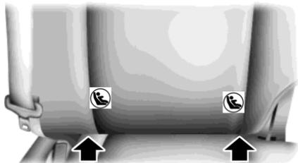
The LATCH anchors are located at the rear section of the rear seat between the cushion and seatback below the symbols as shown. Follow the child seat manufacturer's instructions to properly install a child seat with LATCH attachments.
