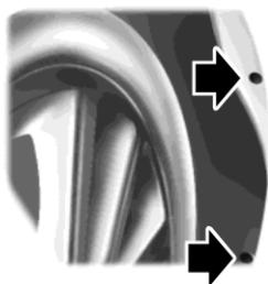
3. At the wheel well, remove the fasteners from the splash shield, then pull the splash shield back to gain access to the bulbs.
