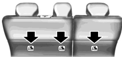
2. Locate the correct anchor behind the gap cover for the selected seating position.
