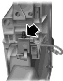
2. Locate the brake shift interlock lever in front of the shifter assembly.
