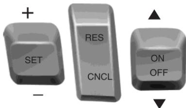
The cruise controls are located on the steering wheel.
