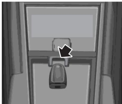
1. Place the new unprogrammed intelligent access key, with the buttons facing down, in the pocket inside of the center console.
