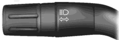
Push the lever forward to switch the high beams on.
