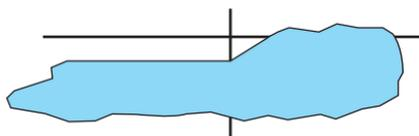
There is a distinct cut-off (change from light to dark) in the left portion of the beam pattern. The top edge of this cut-off should be positioned 2 inches (5 centimeters) below the horizontal reference line.
