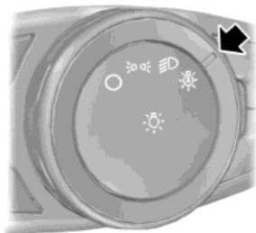
**Note:** If your vehicle is equipped with autolamps, it will have the *windshield wiper activated headlamps*. The windshield wiper activated headlamps turn on within 10 seconds when you switch the windshield wipers on and the lighting control switch is in the autolamps position. They will turn off approximately 60 seconds after you switch the windshield wipers off.
