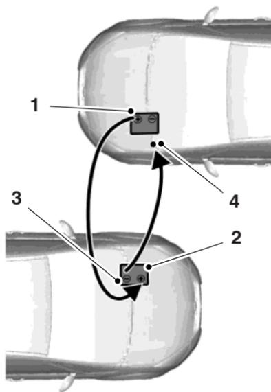
1. Connect the positive (+) jumper cable to the positive (+) terminal of the discharged battery.
