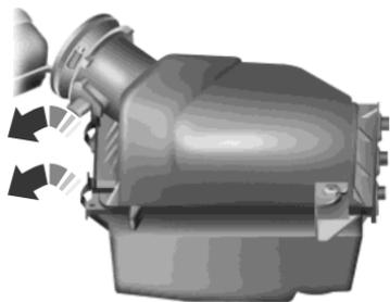
1. Release the clamps that secure the air filter housing cover.
