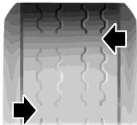
When the tread is worn down to 1/16th of an inch (2 millimeters), tires must be replaced to help prevent your vehicle from skidding and hydroplaning. Built-in treadwear indicators, or wear bars, which look like narrow strips of smooth rubber across the tread will appear on the tire when the tread is worn down to 1/16th of an inch (2 millimeters).
