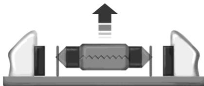
3. Carefully pull the bulb straight out from the lamp assembly.
