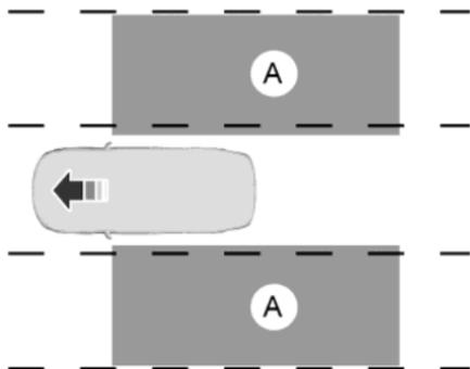
CTA warns the driver of vehicles approaching from the sides when the transmission is in R (Reverse).
