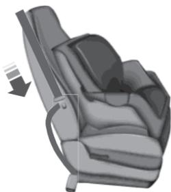
2. Pull down on the shoulder belt and then grasp the shoulder belt and lap belt together.
