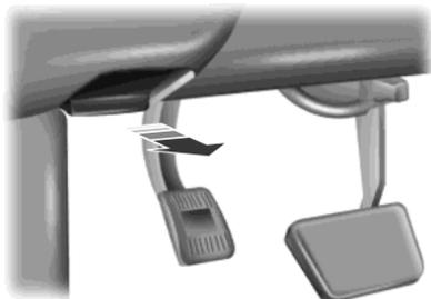
1. Inside the vehicle, pull the hood release handle located under the bottom of the instrument panel near the steering column.
