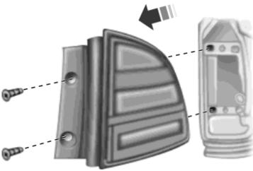
2. Remove the two bolts from the lamp assembly.
