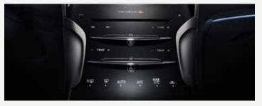
You and your front passenger can press independent controls to adjust the air temperature on each side of the vehicle. To return to one temperature, hold down the **AUTO** button for more than two seconds. The passenger setting then switches to the driver's set temperature.
