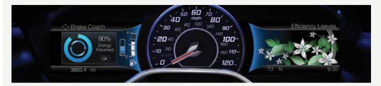
The **Brake Coach** appears in the display after the vehicle has come to a stop, and coaches you to maximize the amount of energy that can be returned through the regenerative braking system.
