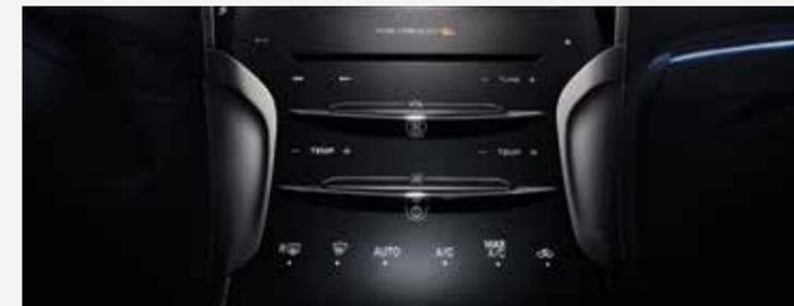
You and your front passenger can press independent controls to adjust the air temperature on each side of the vehicle. To return to one temperature, hold down the **AUTO** button for more than two seconds. The passenger setting then switches to the driver's set temperature.
