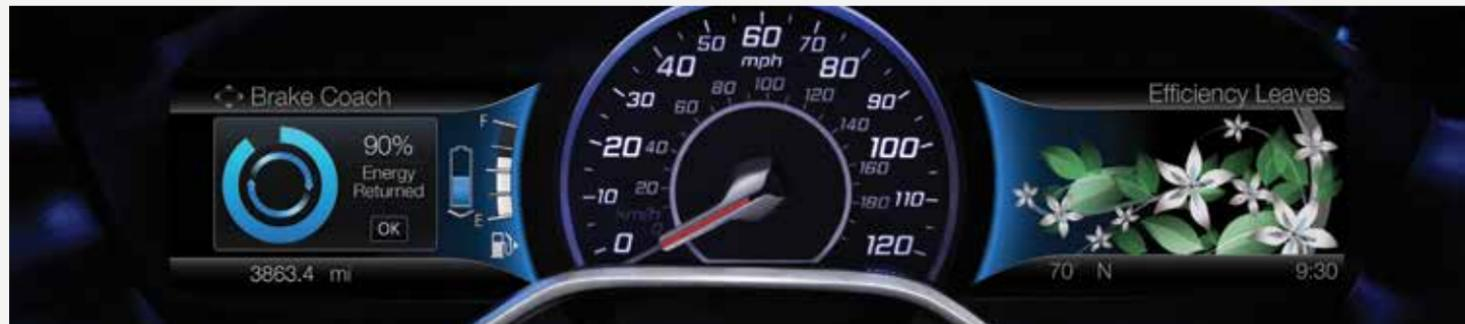
The **Brake Coach** appears in the display after the vehicle comes to a stop, and coaches you to maximize the amount of energy that can be returned through the regenerative braking system.
