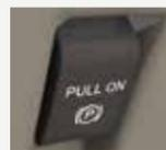
The operating switch (P) replaces the conventional handbrake. The location of the switch is to the left of the steering column. To use, pull the switch up. The brake system warning lamp lights to confirm that you applied the electric parking brake.
