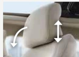
You can adjust your vehicle's front-row head restraints. Pull up to raise the head restraint. To lower, press the head restraint down while pressing and holding the guide sleeve adjust/release button. Tilt the head restraint forward for additional comfort by gently pulling the top of the head restraint.
