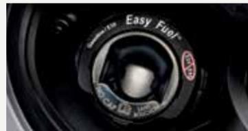
With this system, you simply open the fuel door, insert the nozzle and begin fueling. It is self-sealing and therefore protected against dust, dirt, water, snow and ice. Wait 10 seconds from the time the refueling nozzle is shut off until you remove the nozzle from the vehicle
