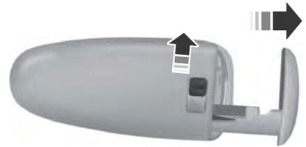
Slide the release on the back of the transmitter, then pull the blade out.
