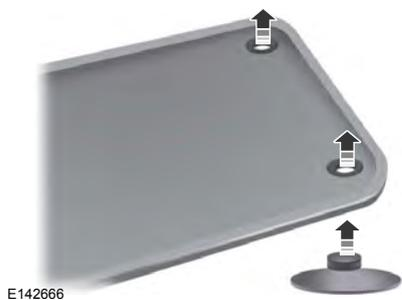
To install floor mats, position the floor mat so that the eyelet is over the retention post and press down to lock in.
