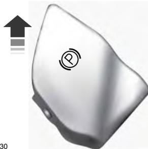
Pull the switch up to apply the electric parking brake.
