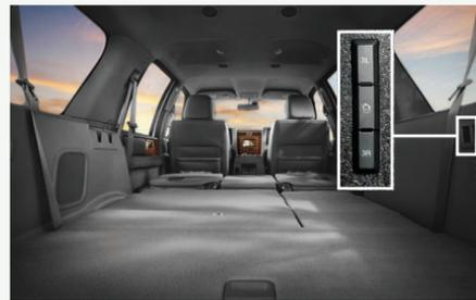
The 60/40 split-folding bench seat uses a power-activated seatback release. The three-button system allows you to fold both sides down at once, or fold each side down independently for more flexibility. The controls are on the right-hand rear quarter trim panel, accessible from the liftgate area.
