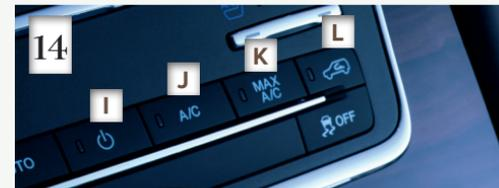
**K. MAX A/C:** Press to maximize cooling. Recirculated air flows through the instrument panel vents, air conditioning automatically turns on, and the fan automatically adjusts to the highest speed.
