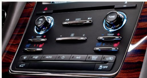
To use the heated seats, press the right side of the button . For cooled seats, press the left side of the button . Press the desired button repeatedly to cycle through the settings, from the highest to the lowest, and then off. More indicator lights mean higher settings.
