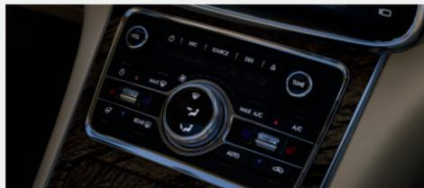
The remote start feature allows you to pre-condition your vehicle's interior. When you set the climate control system to **AUTO**, it automatically adjusts the cabin temperature during a remote start if the remote start climate control settings are set to **AUTO** in the information display.
