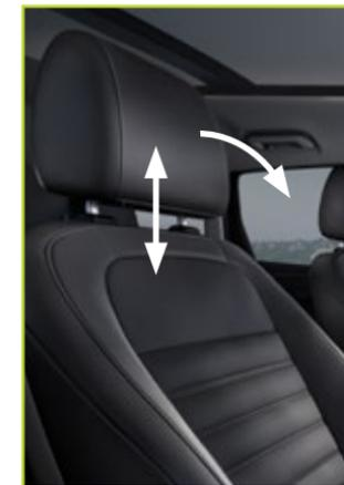
Tilt the head restraint forward for additional comfort by gently pulling the top of the head restraint. Once it is in the forward-most position, tilting it forward again releases it to the upright position.
