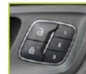
Use this feature to program and recall the positions of the driver seat and power mirrors. The controls are on the driver door. To program position **1**, switch on the ignition, and press and hold the **1** button until you hear a tone.
