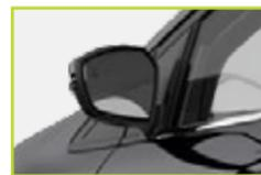
BLIS aids you in detecting vehicles that enter into your blind spot zone. Cross traffic alert warns you of vehicles approaching from the sides when the transmission is in reverse (R).
