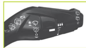
Adjust the wiper lever and its controls to operate the front and rear wipers.
