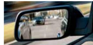
BLIS uses radar sensors to help you determine if a vehicle may be in your blind spot zone. Cross Traffic Alert is designed to warn you of vehicles approaching from the sides when the transmission is in reverse (R).
