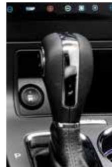
Use this feature to change gears manually. To use, move the gearshift lever from drive (D) to sport (S). Depending on your vehicle, use the toggle on the side of your gearshift lever or paddle shifters on your steering wheel to make shifts.
