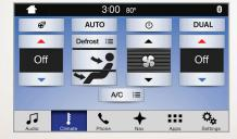
Touch the **Climate** icon on the touchscreen to access climate control features, including the temperature, airflow direction, fan speed and other climate features for you and your front passenger. Say "Climate set temperature to 72 degrees" and SYNC 3 makes the adjustment.
