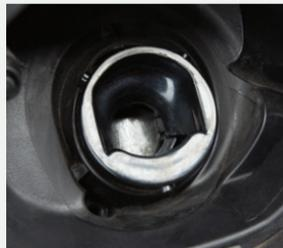
If you are refilling your tank from a fuel container, make sure you use the fuel filler funnel included with your vehicle. Using an aftermarket funnel may not work with the capless system and could cause damage to your vehicle. For more information and for your fuel filler funnel location, please see the **Fuel and Refueling** chapter of your **Owner's Manual**.
