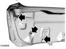
2. Turn the bulb holder counterclockwise and remove it.
