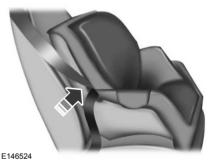
5. To put the retractor in the automatic locking mode, grasp the lap portion of the inflatable seatbelt and pull upward until you pull all of the belt out.
