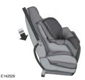
After positioning the child safety seat in the proper seating position, pull down on the shoulder belt and then grasp the shoulder belt and lap belt together behind the belt tongue.
