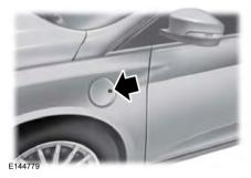
**Note:** Do not force the charge port door open or closed. Forcing the door open or closed will damage the charge port.
