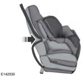
While holding the shoulder and lap belt portions together, route the tongue through the child restraint according to the child restraint manufacturer's instructions. Be sure the belt webbing is not twisted.
