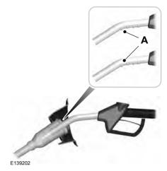
3. Insert the fuel pump nozzle up to the first notch on the nozzle A. Keep it resting on the cover of the fuel tank filler pipe opening.
