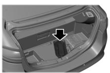
Your vehicle is equipped with a standard 120 volt convenience cord located under the luggage compartment floor covering. The 120 volt convenience cord allows you to charge the high voltage battery using a standard 120 volt household outlet.
