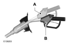
4. Hold the fuel pump nozzle in position B when refueling. Holding the fuel nozzle in position A can affect the flow of fuel and shut off the fuel nozzle before the fuel tank is full.
