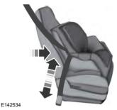
10. Before placing the child in the seat, forcibly move the seat forward and back to make sure the seat is securely held in place. To check this, grab the seat at the belt path and attempt to move it side to side and forward and back. There should be no more than 1 in (2.5 cm) of movement for proper installation.
