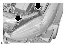
5. Remove the two screws securing the headlamp using a flat-bladed screwdriver.
