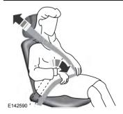
Pregnant women should always wear their seatbelt. Position the lap belt portion of a combination lap and shoulder belt low across the hips below the belly and worn as tight as comfort allows. Position the shoulder belt to cross the middle of the shoulder and the center of the chest
