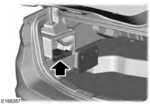
The 12V battery is located in the left-hand side of the luggage compartment. Remove the door to gain access to the battery.
