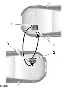
**Note:** In the illustration, the bottom vehicle represents the booster vehicle.
