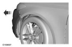
8. Separate the front bumper cover from the fender by gently pulling the front bumper cover to the outside of the vehicle 1.2 in (3 cm).
