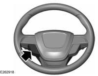
The cruise controls are on the steering wheel. A more detailed graphic is in the Steering Wheel information. See **Cruise Control** (page 73).
