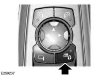
Press the control to lock or unlock the rear window controls. It illuminates when you lock the rear window controls.
