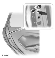
The childproof locks are located on the rear edge of each rear door and must be set separately for each door.
