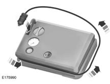
Wrap the power cord around the housing and stow the accessory power plug into its storage area.
