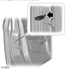
If the central locking function does not operate, lock the doors individually using the key in the position shown. On the left-hand side, turn the key clockwise to lock. On the right-hand side, turn the key counterclockwise to lock.
