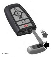
Push the release button and pull the key blade out.
