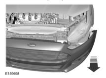
9. From the front of the vehicle, gently pull the front bumper cover forward 4 in (10 cm) by grasping it next to the headlamp to be serviced and in the lower front of the wheel opening.
