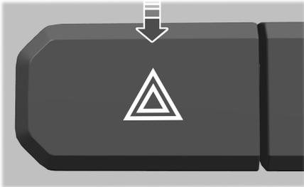
The hazard flasher control is located on the instrument panel. Use it when your vehicle is creating a safety hazard for other motorists.
