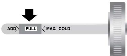
**Note:** The power steering cap has both a cold and hot indicator on the dipstick.
