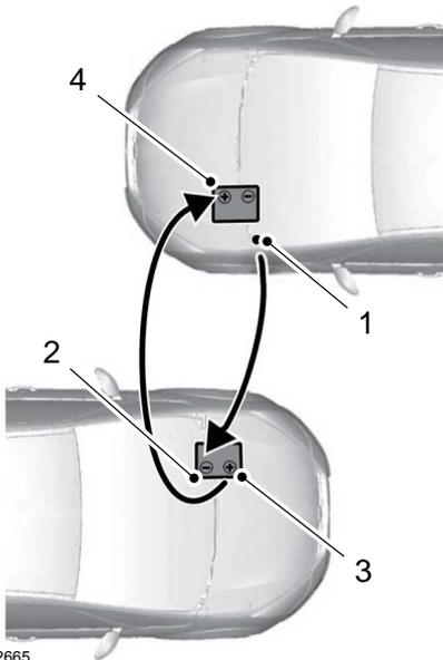
1. Remove the negative (-) jumper cable from the disabled vehicle.
