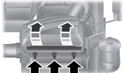
1. Loosen the latches that secure the air filter cover in place.
