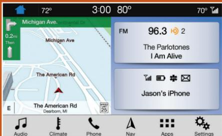
The SYNC 3 system allows you to interact with a variety of features using the touchscreen and voice commands. By integrating with your *Bluetooth* wireless technology-enabled phone, the touchscreen provides easy integration with many of your vehicle's features.
