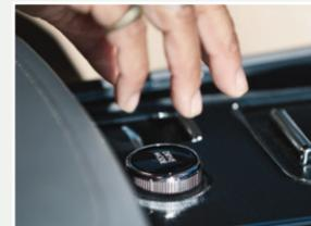
**Note:** If the electric parking brake warning lamp stays on, then the electric parking brake did not automatically release. You must release the electric parking brake using the switch.
