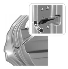
A child safety lock is on the rear edge of each rear door. You must set the child safety lock separately on each door.
