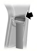
To adjust the shoulder belt height, squeeze the button and slide the height adjuster up or down. Release the button and pull down on the height adjuster to make sure it is locked in place.
