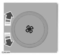
Turn the control to adjust the volume of air circulated in the vehicle.
