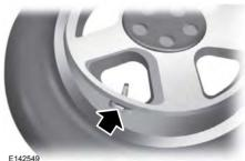
E142649 **Note:** Each road tire is equipped with a tire pressure sensor located inside the wheel and tire assembly cavity. The pressure sensor is attached to the valve stem. The pressure sensor is covered by the tire and is not visible unless the tire is removed. Take care when changing the tire to avoid
