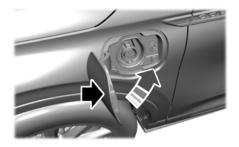
4. Press the center right edge of the charge port door to close.
