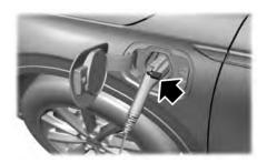
**Note:** You will need a padlock or a combination lock with a shackle diameter of 0.2 in (5 mm) or less and the straight portion of the shackle of 1.0 in (25.4 mm) of length or more.
