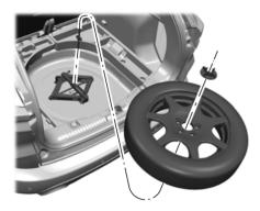
Turn the jack hex nut drive screw counterclockwise to detach the lug wrench from the jack. This lowers the jack and releases the mechanical lock.
