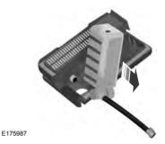
4. Rotate the sealant canister up 90 degrees and pull away from casing/housing to remove.
