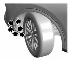
2. Remove the six lower splash shield push pins and pull the splash shield back.
