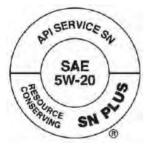
An oil that displays this symbol conforms to current engine, emission system and fuel economy performance standards of ILSAC.
