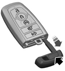
1. Push the release button and pull the key blade out.
