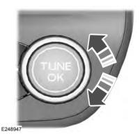
In radio mode, turn to search through the radio frequency band.
