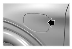
**Note:** Do not force the charge port door open or closed. Forcing the door open or closed will damage the charge port.
