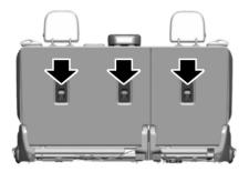
2. Locate the correct anchor on the back panel of the rear seat for the selected seating position. The anchors are labeled with the tether strap symbol.
