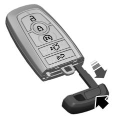
Push the release button and pull the 1. key blade out.
