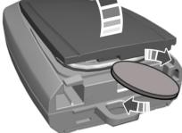
2. Twist a thin coin under the tab hidden behind the key blade head to remove the battery cover.
