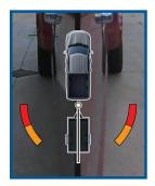
The hitch angle graphic display shows you a small, top-view representation of your truck and trailer.
