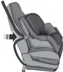
3. While holding the shoulder and lap belt portions together, route the tongue through the child restraint according to the child restraint manufacturer's instructions. Make sure you did not twist the belt webbing.
