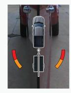
The hitch angle graphic display shows you a small, top-view representation of your vehicle and trailer.
