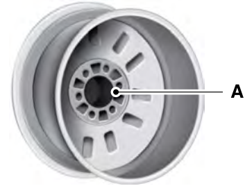
A Hub pilot bore.
