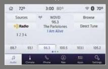
To set a new preset, tune to the station and then press and hold one of the preset buttons. The audio mutes briefly while the system saves the station and then returns. To access additional presets, swipe left.
