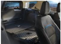
stowed To unfold the seat backrest, pull the seat backrest up to unfold it. See the Seats chapter of the Owner's Manual for more information.
