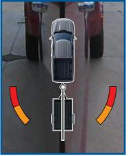
The hitch angle graphic shows you a small, top-view representation of your vehicle and trailer.
