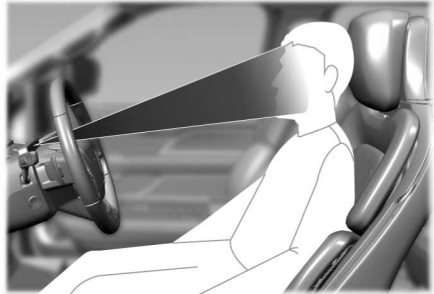
Appropriate position, camera can see the face.
