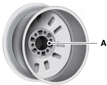
A Hub pilot bore.
