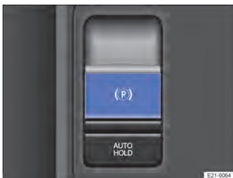
Fig. 110 In the centre console: button for the electric parking brake.
