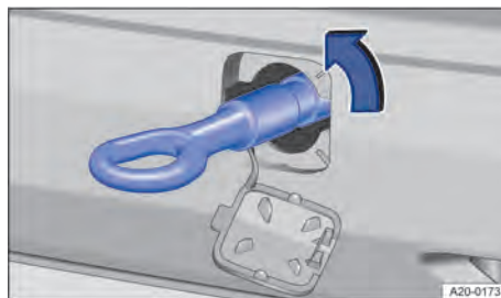
Fig. 191 In the rear right bumper: screwing in the towing eye.
