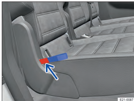
Fig. 64 Second row of seats: marking indicating that the seat backrest is not engaged properly.
