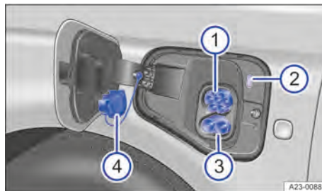
Fig. 157 Behind the charging socket flap at the front left: charging socket.
