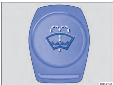
Fig. 197 In the engine compartment: cap of washer fluid reservoir
