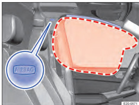
Fig. 34 On the left-hand side of the vehicle: Location and deployment zone of the curtain airbag (2-seater).
