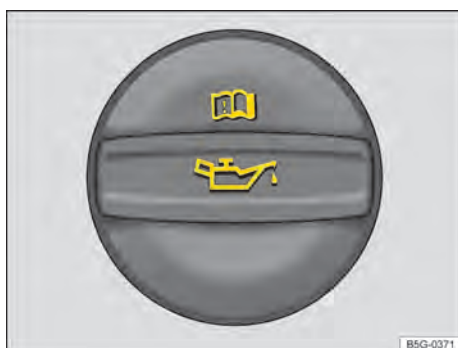
Fig. 199 In the engine compartment: engine oil filler opening cap (illustration).
