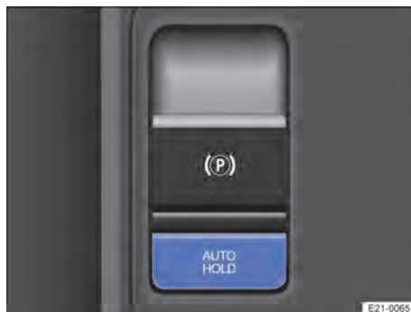
Fig. 112 In the centre console: button for Auto Hold.
