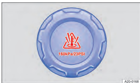
Fig. 200 In the bonnet space: cap of the coolant expansion tank.
