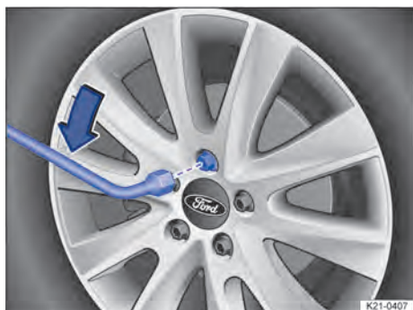
Fig. 212 Loosening the wheel bolts.
