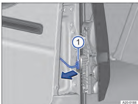
Fig. 176 On the tail lamp cluster: disconnecting the connector.
