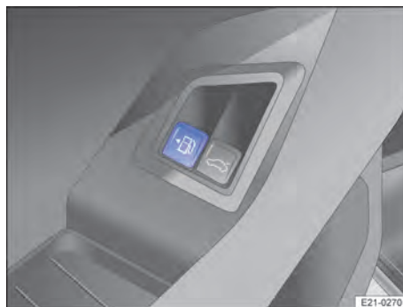
Fig. 150 In the driver door: release button for the tank flap.
