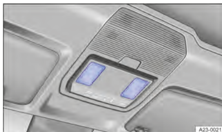
Fig. 80 In the roof console: touch-sensitive reading lights.
