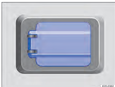
Fig. 127 On the rear centre console or on the partition to the load compartment: 230-volt socket with earthing contact with cover flap (illustration).
