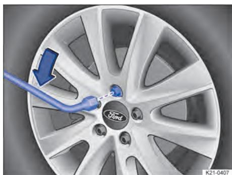
Fig. 216 Unscrew the wheel bolts with the wheel wrench.
