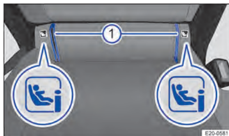
Fig. 39 On the rear seats: Marking variants identifying the ISOFIX anchor points for child seats.
