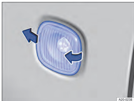
Fig. 173 On the side of the vehicle: removing the direction indicator repeater.
