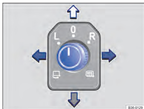
Fig. 86 In the driver door: rotary knob for the exterior mirrors
