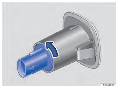
Fig. 174 Replacing the bulb in the direction indicator repeater.
