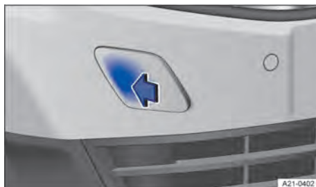
Fig. 188 In the front right bumper: Remove the cover.
