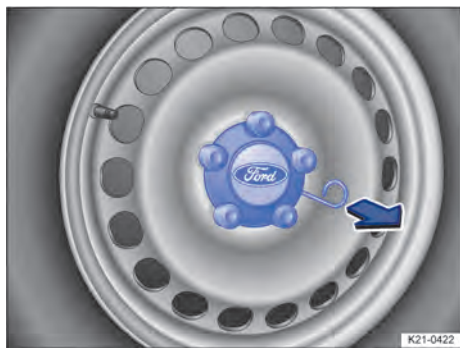
Fig. 209 Pulling off the centre wheel trim (illustration).
