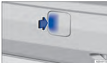
Fig. 190 In the rear right bumper: Remove the cover.
