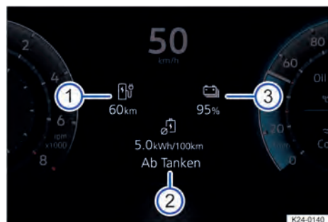
Fig. 13 In the main display area of the digital instrument cluster: charge level and range (illustration).
