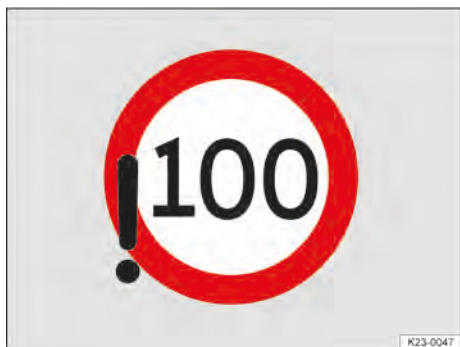
Fig. 25 On the instrument cluster display: detected violation of maximum permitted speed (illustration).
