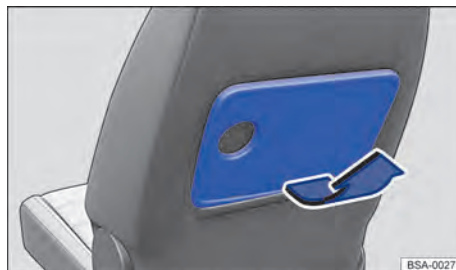
Fig. 124 Front seat: setting up the folding table.
