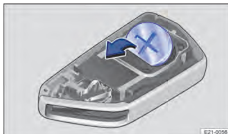
Fig. 51 Vehicle key: changing the button cell.
