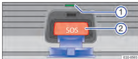
Fig. 47 Control for emergency call: indicator lamp and button.
