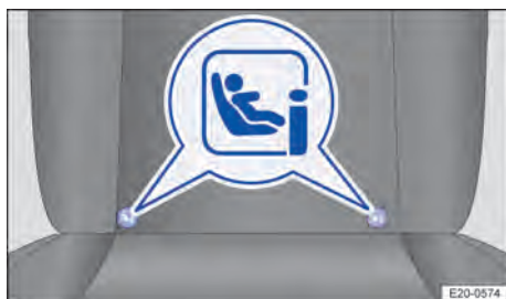
Fig. 38 Front passenger seat: Marking variants identifying the ISOFIX anchor points for child seats.
