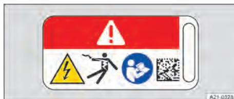
Fig. 153 Warning sign on high-voltage components.
