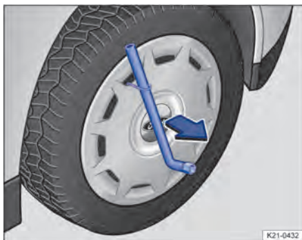
Fig. 210 Pulling off the wheel cover (illustration).
