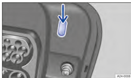
Fig. 159 Behind the charging socket flap: Charging process display.
