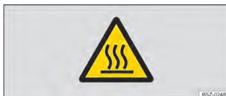
Fig. 155 Warning sign for hot surfaces on the battery charger.
