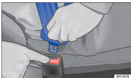
Fig. 24 Removing the latch plate from the buckle
