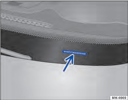
Fig. 227 In the windscreen: vehicle identification number.
