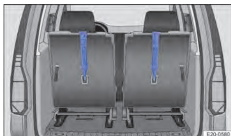
Fig. 47 Third seat row: top tethers fitted (depending on equipment).
