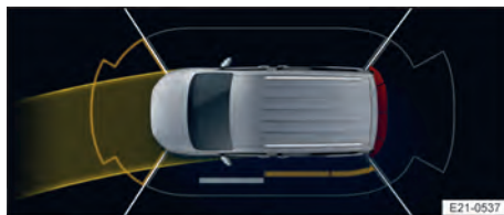
Fig. 125 On the Infotainment system: obstacle detection and steering wheel angle for parking sensors (illustration).
