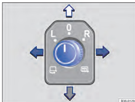
Fig. 91 In the driver door: rotary knob for the exterior mirrors
