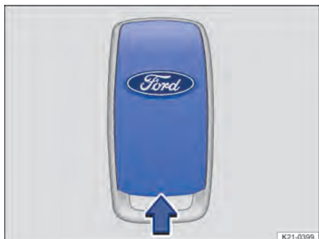
Fig. 95 Replace the button cell in the remote control.
