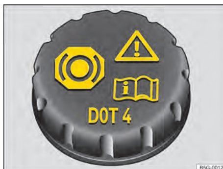
Fig. 201 In the engine compartment: cap on the brake fluid container
