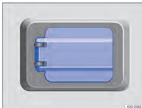
Fig. 144 On the rear centre console or on the partition to the luggage compartment: 230-volt socket with earthing contact with cover flap (illustration).
