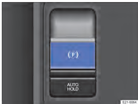
Fig. 121 In the centre console: button for the electric parking brake.
