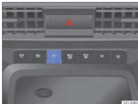
Fig. 126 In the centre console: touch panel for parking functions.
