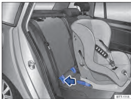
Fig. 43 Illustration: fitting an ISOFIX child seat with the attachment arms.
