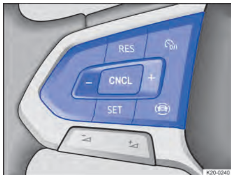
Fig. 107 Left-hand side of the multifunction steering wheel.
