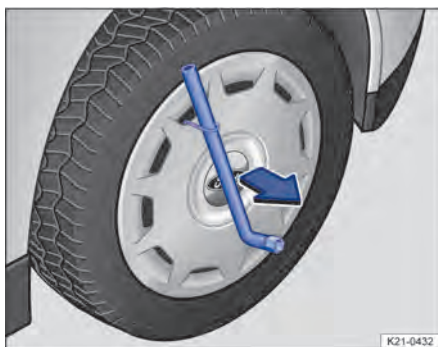
Fig. 211 Removing the wheel cover.
