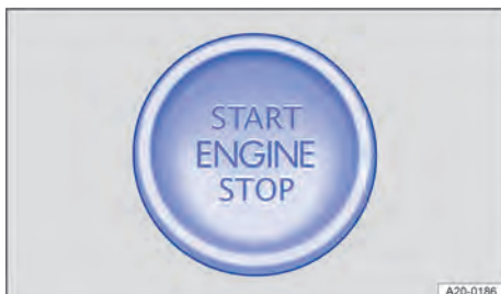
Fig. 101 In the lower section of the centre console: Push button ignition switch for starting the engine.
