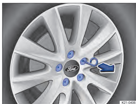
Fig. 212 Removing the wheel bolt caps
