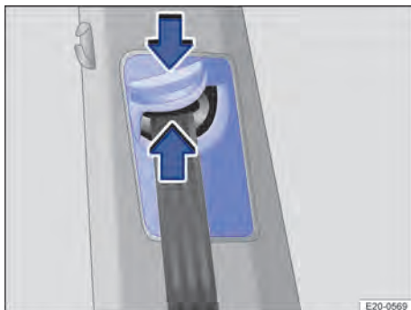
Fig. 27 Next to the front seats: seat belt height adjuster.
