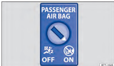
Fig. 32 On the front of the dash panel: key switch for disabling and enabling the front airbag on the front passenger side
