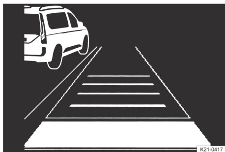
Fig. 109 In the instrument cluster display: slower vehicle detected in the left-hand lane (illustration).
