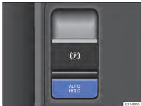
Fig. 122 In the centre console: button for Auto Hold.
