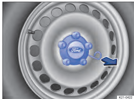
Fig. 210 Pulling off the centre wheel trims.
