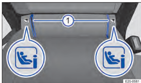
Fig. 41 On vehicle seat in second seat row: marking variants identifying the ISOFIX anchorage points for child seats.
