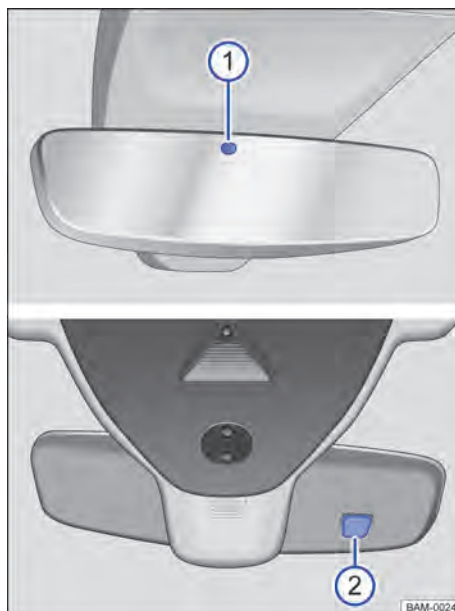
Fig. 89 On the windscreen: automatic anti-dazzle interior mirror.
