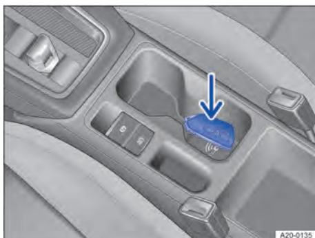
Fig. 102 In the centre console: emergency start function.
