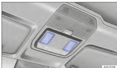
Fig. 85 In the roof console: Touch-sensitive reading lights.
