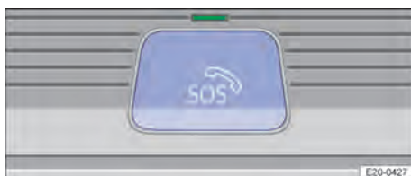
Fig. 49 In the roof console: control for eCall Emergency System (behind button cover).
