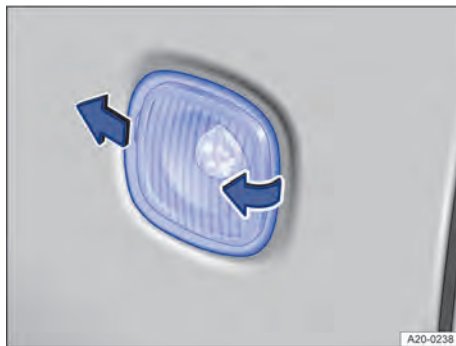
Fig. 176 On the side of the vehicle: removing the turn signal repeater.
