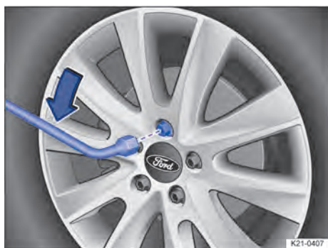
Fig. 218 Wheel change: Unscrew the wheel bolts with the wheel wrench.
