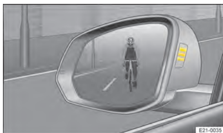
Fig. 124 In the exterior mirror housings: visual display of exit warning system
