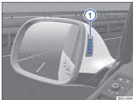
Fig. 120 In the exterior mirror housings: visual displays of Blind Spot Assist.
