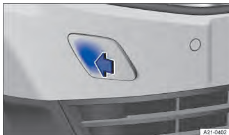
Fig. 189 In the front bumper on the right: removing the cover.
