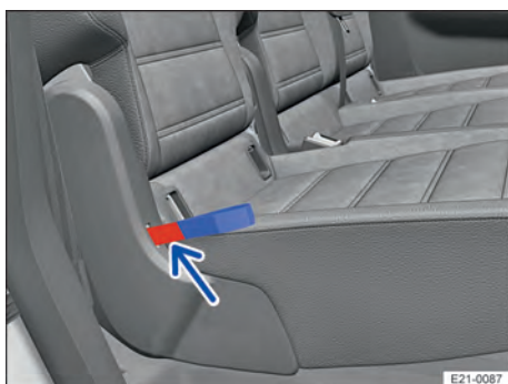
Fig. 66 Second row of seats: Marking indicating that the seat backrest is not engaged properly.
