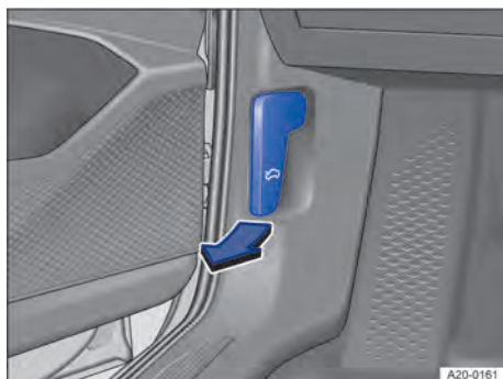
Fig. 191 In the footwell on the left side: bonnet release lever (illustration).
