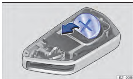
Fig. 54 Vehicle key: changing the button cell.
