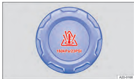
Fig. 199 In the engine compartment: coolant expansion tank cap
