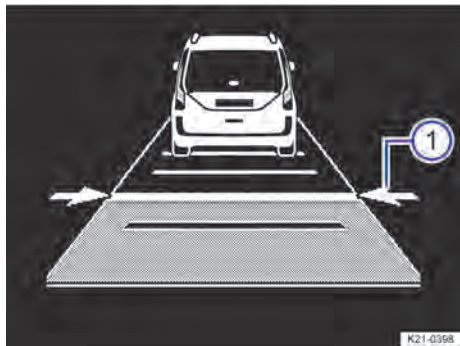
Fig. 115 On the display of the analogue instrument cluster: set distance ①, Adaptive Cruise Control is controlling the vehicle (illustration).
