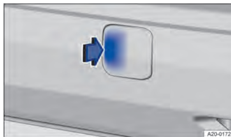
Fig. 187 In the rear bumper on the right: removing the cover.
