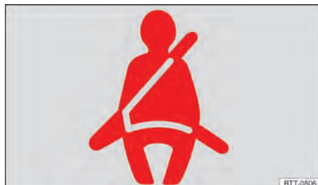
Fig. 21 On the instrument cluster display: warning lamp.
