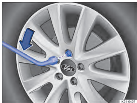
Fig. 214 loosening the wheel bolts.
