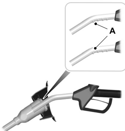
3. Insert the fuel pump nozzle up to the first notch on the nozzle A. Keep the fuel pump nozzle resting on the fuel tank filler pipe.
