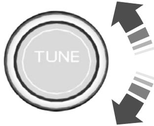
3. Rotate the control to change the frequency.
