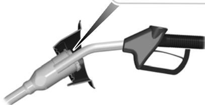
4. Hold the fuel pump nozzle in position B when refueling. Holding the fuel pump nozzle in position A can affect the flow of fuel and shut off the fuel pump nozzle before the fuel tank is full.
