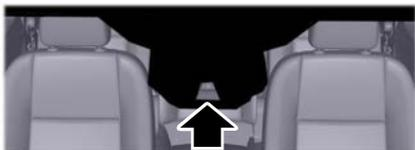
The camera is mounted behind the interior mirror.
