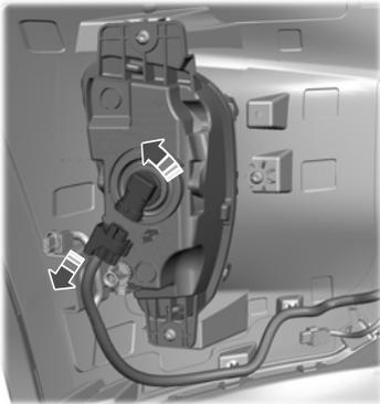
3. Disconnect the bulb electrical connector.
