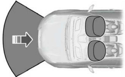
The airbag will deploy during significant frontal and near frontal collisions. The airbag will inflate within a few thousandths of a second and deflate on contact with the occupant, thus cushioning forward body movement. During minor frontal collisions, overturns, rear collisions and side collisions, the airbag will not deploy.
