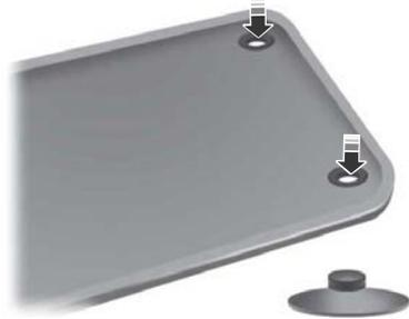
To install floor mats that have eyelets, position the floor mat eyelet over the retention post and press down to lock in position. Repeat for all eyelets on the floor mat.
