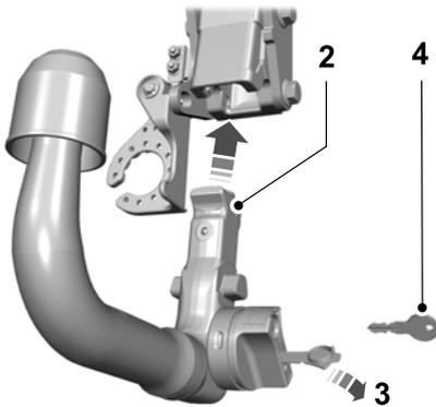
2. Fully insert the tow ball arm until it engages. Do not hold the handwheel.
