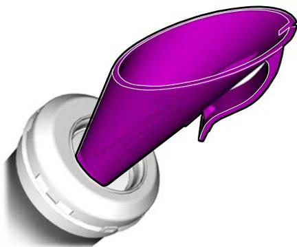
2. Fully insert the fuel filler funnel into the fuel filler inlet.
