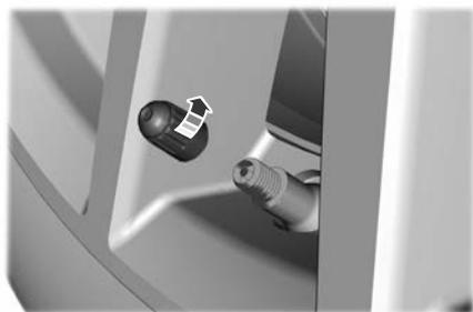
1. Remove the valve cap from the tire valve.
