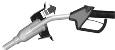
3. Insert the fuel pump nozzle up to the first notch on the nozzle A. Keep it resting on the cover of the fuel tank filler pipe opening.
