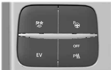
Your vehicle contains selectable electric vehicle (EV) modes. Press the button on the center console to change the mode. EV Now and EV Later modes are only available when you have electric-only driving range available.
