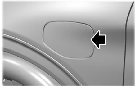
**Note:** Do not force the charge port door open or closed. Forcing the door open or closed will damage the charge port.
