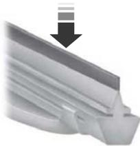
Run the tip of your fingers over the edge of the blade to check for roughness.
