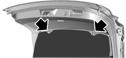
3. Insert the retaining clips into the liftgate trim panel.
