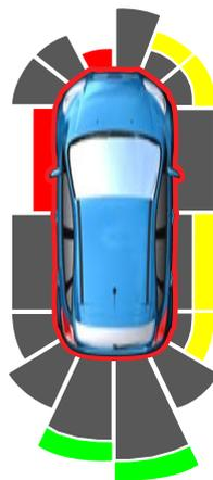
The system uses red, yellow and green highlights that appear on top of the video image when any of the sensing systems detect an object.
