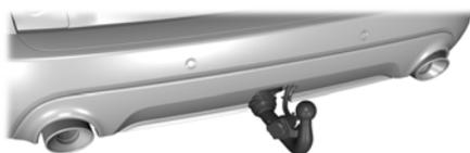
2. Press the button again within four seconds to deploy the tow ball arm to the released position. The tow ball arm moves into the tow position.
