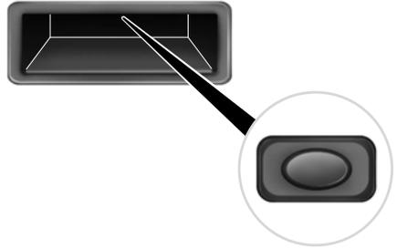
Press the control button to unlatch the liftgate and then lift to open.
