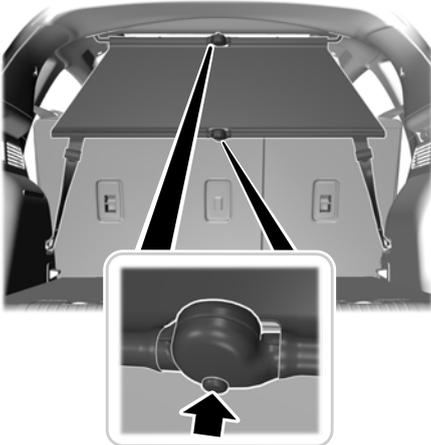
4. Push the release buttons to fold the cargo net.
