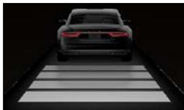
The selected gap appears in the instrument cluster display as shown by the bars in the image.
