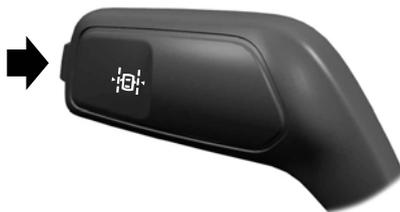
Press the button on the direction indicator stalk.
