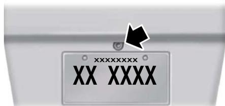
The camera is located on the liftgate.
