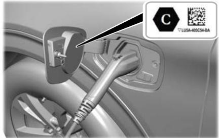
4. Plug the charge station coupler into the the charge port on your vehicle.
