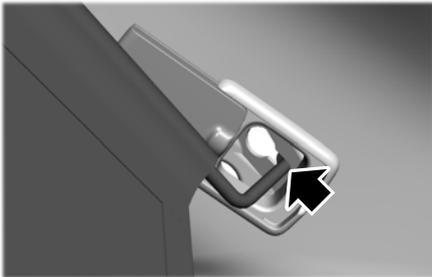
1. Push the ends of the upper bar toward each other and insert them into the retainers on the headliner. Push the bar forward into the narrow section of the retainers.
