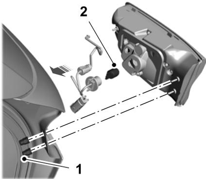
1. Remove the screws with a flathead screwdriver and pull the lamp assembly away from the vehicle.
