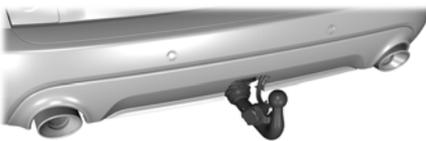
3. Press the button again within four seconds to retract the tow ball arm to the released position. The tow ball arm moves into the stowed position.
