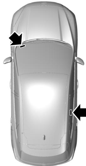
The vehicle identification number is stamped into the floor panel on the right-hand side, beside the rear seat. It is also shown on the left-hand side of the instrument panel.
