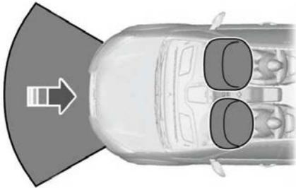
The airbag is designed to deploy during a significant frontal or near-frontal crash. The airbag inflates within a few thousandths of a second cushioning forward body movement and deflates on contact with the occupant. The airbag is not designed to deploy during a minor frontal crash, rear crash, side crash or a vehicle rollover.
