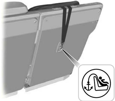
Top tether anchor points are on the back of the rear seat.
