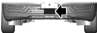
The radar sensor is in the lower grille.
