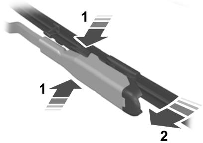
1. Lift the wiper arm and then press the wiper blade locking buttons together.
