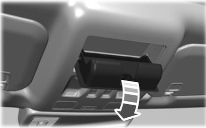
Press near the rear edge of the door to open it.
