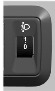
Rotate the control in accordance with your vehicle load to prevent you from distracting other road users when the headlamps are on.
