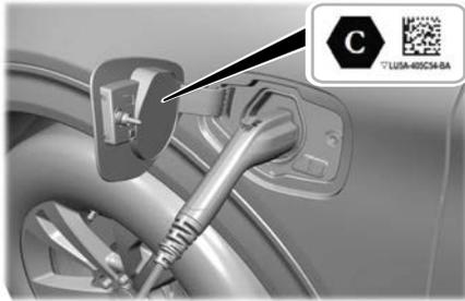
4. Plug the charge coupler into the charge port on your vehicle.
