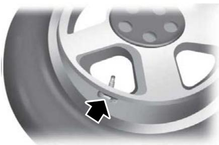
**Note:** Each road tire comes with a tire pressure sensor located inside the wheel and tire assembly cavity. The pressure sensor is attached to the valve stem. The pressure sensor is covered by the tire and is not visible unless the tire is removed. Take care when changing the tire to avoid damaging the sensor.
