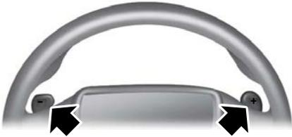
Shift to manual (M) to switch the feature on.
