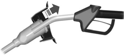
6. When the nozzle shuts off, wait at least 5 seconds, then slightly raise the fuel pump nozzle and slowly remove it.
