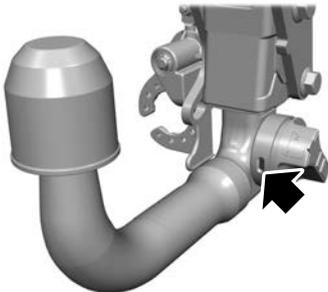
1. The mark on the handwheel is green.
