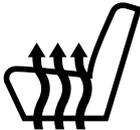
Press the heated seat symbol to cycle through the various heat settings and off. More indicator lights indicate warmer settings.
