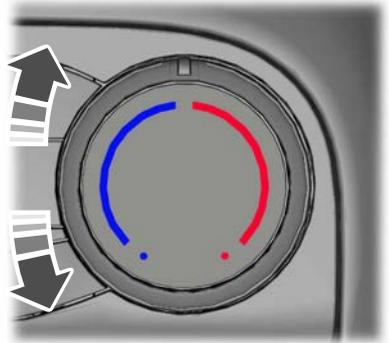
Turn the temperature control counterclockwise for cooler temperature settings.
