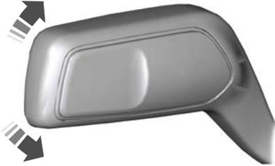
Push the lever up or down to switch the direction indicators on.
