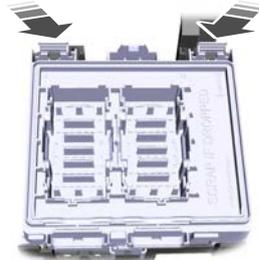
4. Pull both latches toward you and remove the fuse box.
