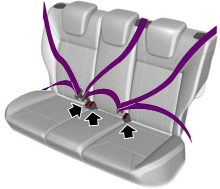
Pull the belt out steadily. It may lock if you pull it sharply or if your vehicle is on a slope.
