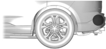
The sensors are behind the rear bumper on both sides of your vehicle.
