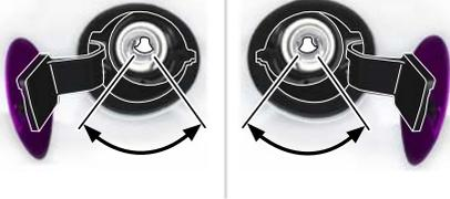
5. Operate the fuel pump nozzle within the area shown.
