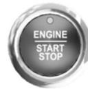
1. Press and hold the push button ignition switch until the engine stops, or press it three times within two seconds.
