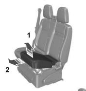
**Note:** Only the inboard seat has a storage compartment.
