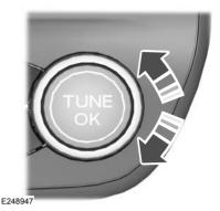
Rotate the control to change radio stations.
