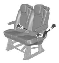
With the seat occupied, lift the recline lever or pull the strap to recline the seat backrest.
