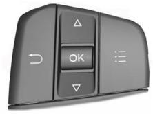
Press the **OK** button to acknowledge and remove some messages from the information display. You need to confirm certain messages before you can access the menus. The information display will automatically remove other messages after a short period of time.
