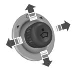
Move the adjustment control in the direction of the arrows to adjust the mirror.
