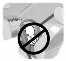
WARNING: Extreme Hazard! Never use a rearward facing child restraint on a seat protected by an active airbag in front of it. Death or serious injury to the child can occur. **WARNING:** You must switch the passenger airbag off when using a rearward facing child restraint on the front seat.
