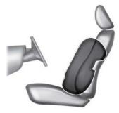
The side airbags are designed to inflate between the door panel and the occupant to enhance the protection in certain crashes.
